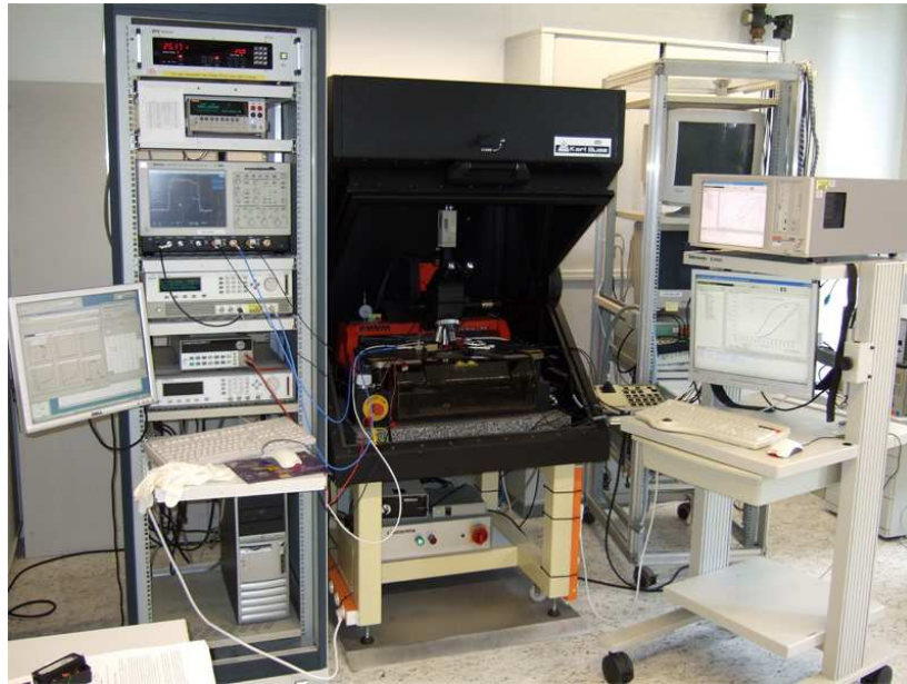
Figure 3.2: Set-up configuration used for the gate oxide time dependent dielectric breakdown experiments and DC characterization.
