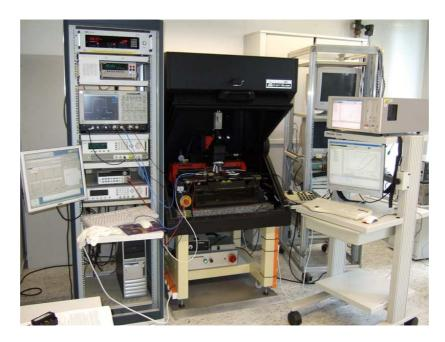
Figure 3.2: Set-up configuration used for the gate oxide time dependent dielectric breakdown experiments and DC characterization.
