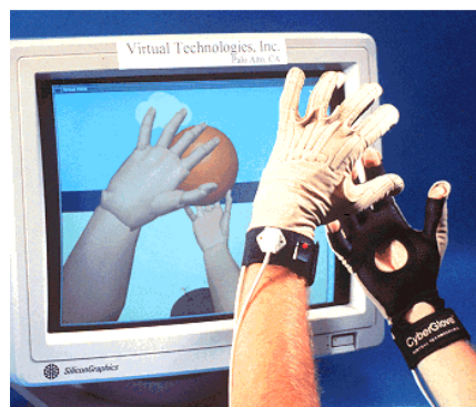
Figure 19 : DataGlove. Illustration extraite de http://www.virtualtechnologiesltd.com/ .
