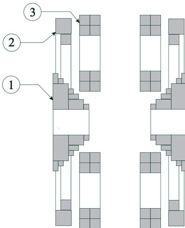
Figure 8.6: Arrangement of individual turns of coils into larger structures (grey rectangles) for improved computation time. Each structure is approximated and modeled as a set of 64 short linear segments.
