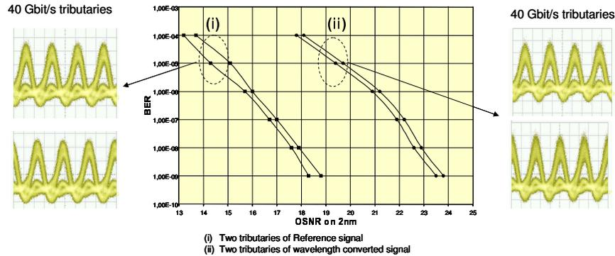
Fig. 3: BER evolution as a function of OSNR measured in 2nm bandwidth
