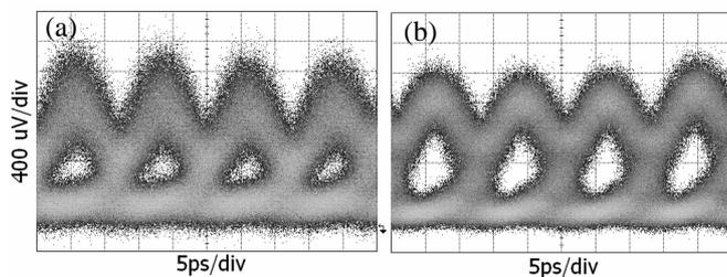
Fig. 6. Eye diagrams of the wavelength converted signal at 80 Gbit/s following (a) RSF and (b) BSF for a power received of -9 dBm relating to a BER of  $\sim 10^{-6}$  and  $10^{-9}$  for RSF and BSF respectively.
