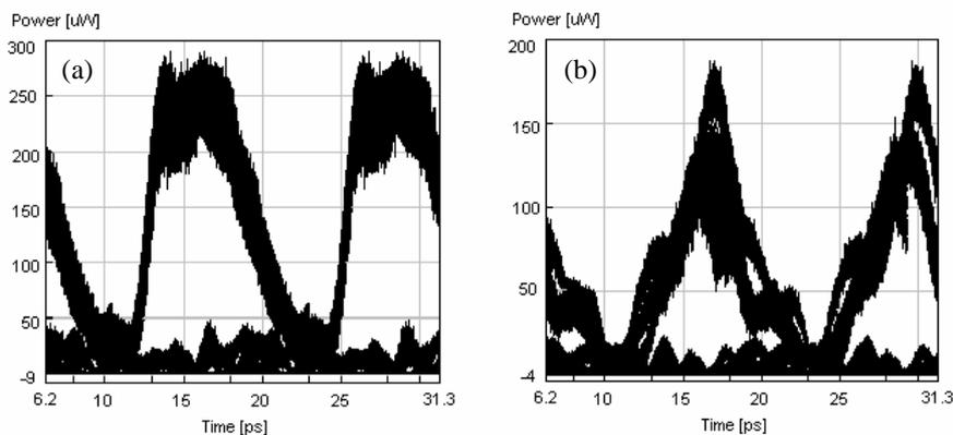
Fig. 10. The 80 Gb/s wavelength converted eye with BSF technique using FROG measurement and modelled by VPI simulation tool (a) before propagation and (b) following 50 km of dispersion compensated fiber span.
