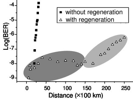
Figure 9 : BER vs distance in a 2R link.
