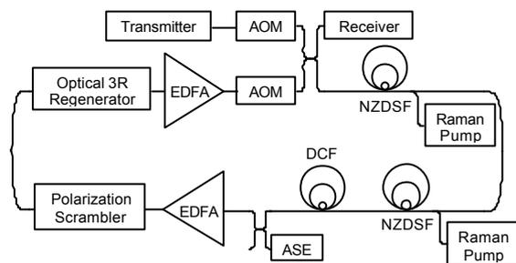
Fig. 3: Recirculating loop.
