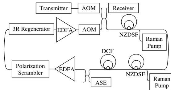
Fig. 1: Recirculating loop.
