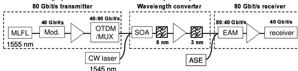
Fig. 1: Experimental setup of wavelength conversion at 80 Gb/s
