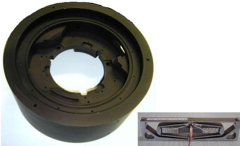
Fig. 3. Photograph of the mechanics of the Tunable Filter of the 3D-NTT. The overall diameter is 30 cm (the useful diameter is 10 cm). The height is 12 cm. The lower right corner insert shows a piezoactuator (not at scale). The three piezoactuators are located at 120^\circ around the central hole. The weight is 16kg (without glass plates and accessories).
