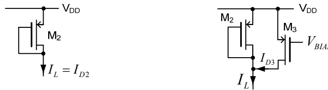
FIG. 5.7: a) Diode connected P-MOS transistor with transconductance g_m , b) Diode connected MOS transistor with decreased transconductance g'_m [80]
