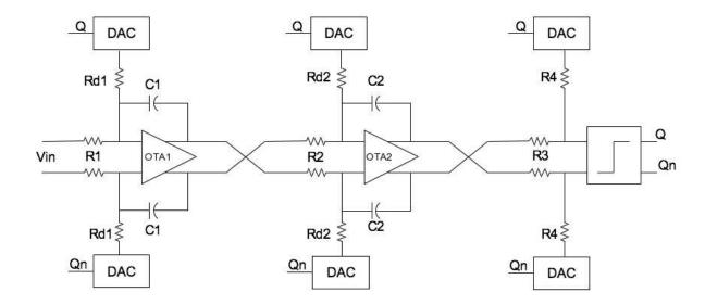
Figure 4.33: CT  $\Sigma\Delta$  Modulator
