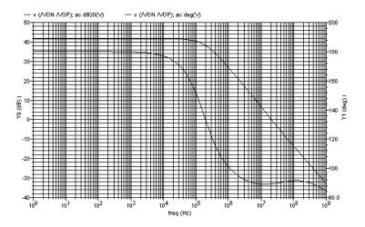
Figure 6.8: First stage pen loop gain.
