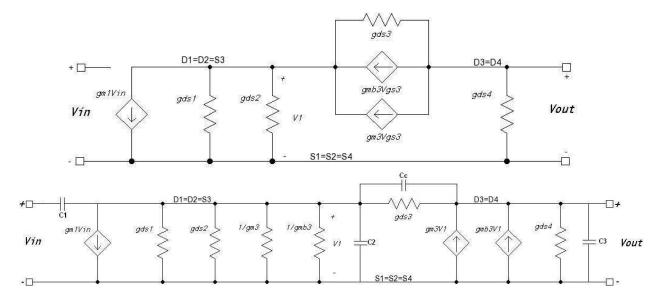
Figure 4.5: OTAs small signal model
