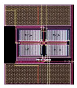
Figure 4.14: Output stage OTA's layout.
