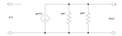
Figure 4.11: Output OTAs small signal model
