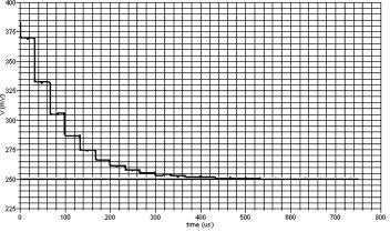
Figure 6.16: First stage output common mode.
