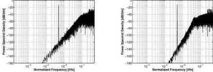
Figure 3.26: Figure (a) to (d): ouput spectrum of first-order to fourth-order single loop single-bit  $\Sigma\Delta$  modulators.
