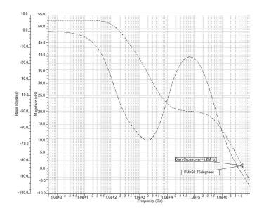
Figure 4.6: First stage open loop gain.
