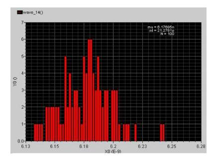
Figure 4.20: IL histogram for a process variation simulation.
