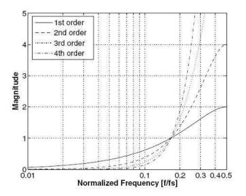
Figure 3.25: Ideal noise transfer functions of  $\Sigma\Delta$  modulator.
