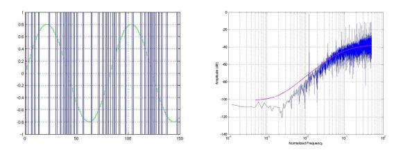
Figure 4.31: Left: Bitstream; Rigth:Bitstream's PSD.
