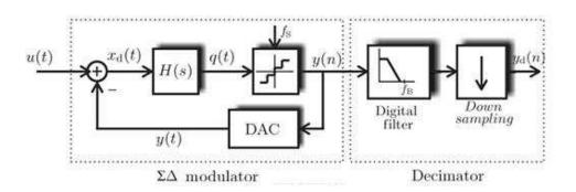
Figure 3.29: Continuous Time  $\Sigma\Delta$  Modulator
