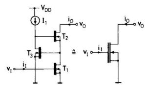
Figure 3.2: Composite transistor. (Taken from [30]).
