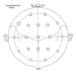
Figure 2.2: EEG electrode 10-20 system. [5]
