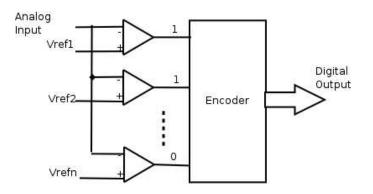
Figure 3.13: Block diagram of a flash ADC
