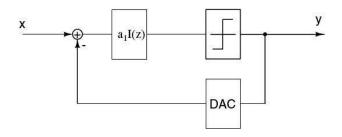
Figure 3.22: The first-order single-loop  $\Sigma\Delta$  modulator.
