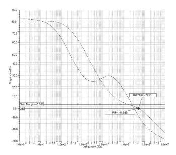
Figure 4.27: Ultra-Low-Voltage amplifier open loop gain.
