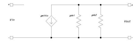
Figure 6.10: Output OTAs small signal model
