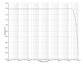
Figure 4.37: ADCs amplifier common mode rejection ratio.
