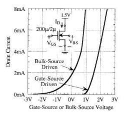
Figure 3.6: Measured linear  $I_D$  Vs.  $V_{BS}$  for the bulk-driven MOSFET and  $V_{GS}$  for the standard MOSFET (Taken from [28]).
