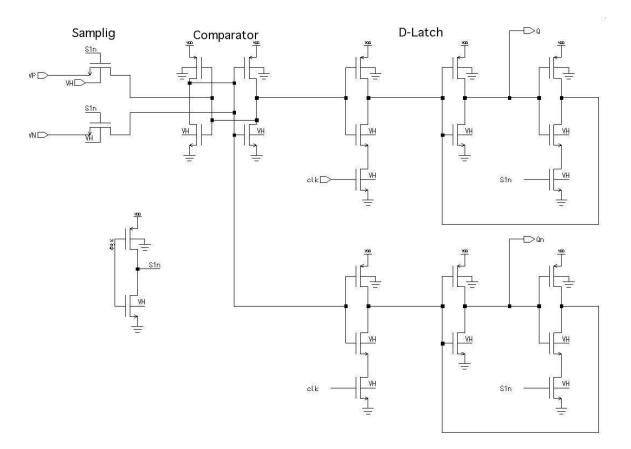
Figure 4.41: Single bit quantizer
