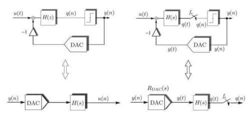
Figure 3.30: Loop filter representation for DT and CT modulators. Left: DT modulator. Right: CT modulator
