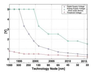
Figure 3.1: Supply voltage and threshold voltage of differents technologies. (Taken from [27])
