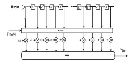
Figure 4.45: FIR diagram.
