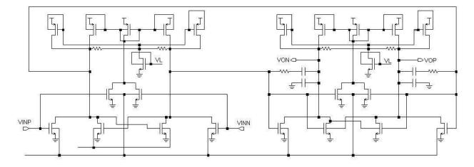
Figure 3.34: Ultra Low Voltage gate-input OTA
