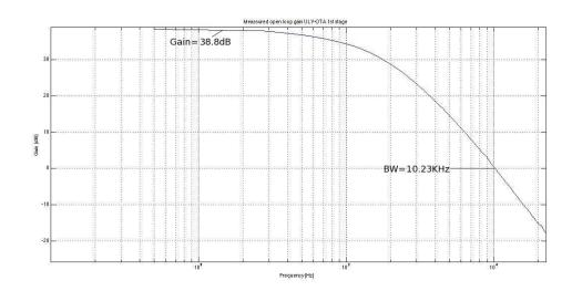
Figure 5.6: ULV-OTA first stage open loop gain.
