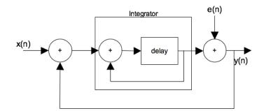
Figure 3.16: Block diagram of a  $\Sigma\Delta$  ADC
