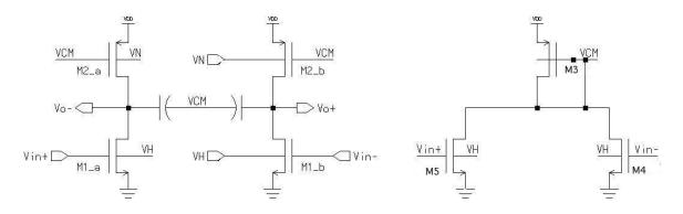
Figure 4.34: Current source amplifier based OTA for a  $\Sigma\Delta$  ADC.
