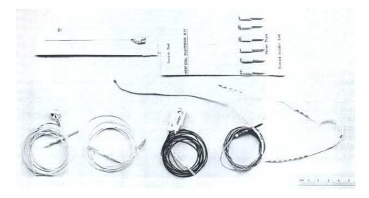
Figure 2.1: Types of electrode for EEG recording. [5]
