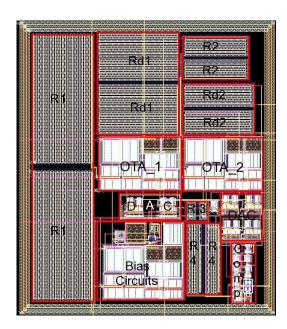
Figure 4.49: CT  $\Sigma\Delta$  Modulator.
