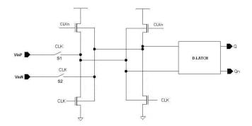
Figure 6.20: Quatizer using D-latch.
