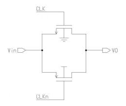
Figure 6.19: Transmission gate circuit used as CMOS switch.
