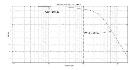
Figure 5.8: ULV-OTA second stage open loop gain.
