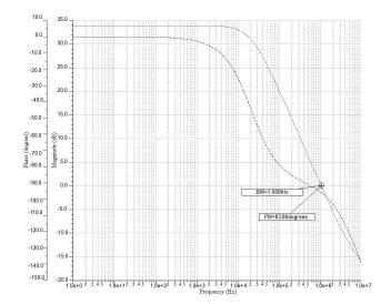
Figure 4.36: ADCs amplifier open loop gain.
