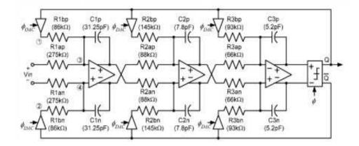
Figure 3.36: CT  $\Sigma\Delta$  Modulator
