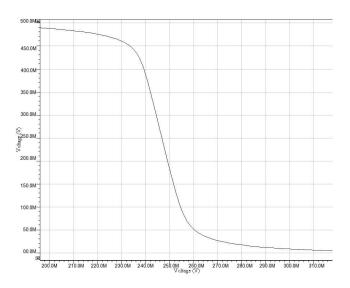
Figure 4.13: Ouput stage output voltage swing.
