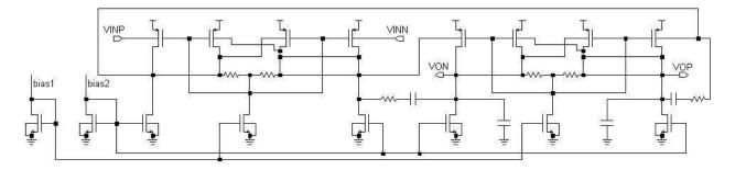
Figure 3.33: Ultra Low Voltage body-input OTA
