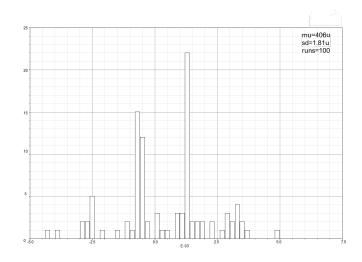
Figure 4.28: Ultra-Low-Voltage amplifier offset.
