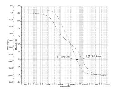
Figure 4.12: Output stage open loop gain.
