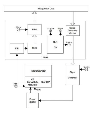
Figure 5.4: Modulator test and information configuration.
