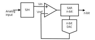
Figure 3.15: Block diagram of a SAR ADC
