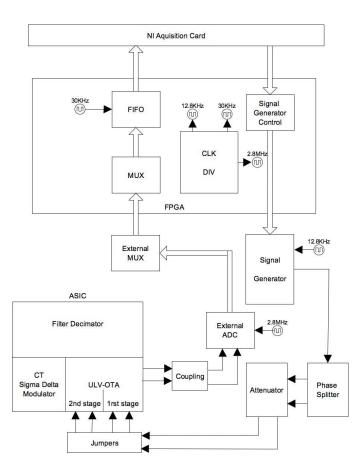
Figure 5.3: ULV-OTA test and information configuration.
