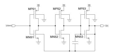
Figure 4.25: Substrate bias circuit.
