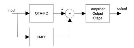
Figure 4.2: ULV OTA block diagram.
