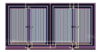
Figure 4.24: Error amplifier layout.
