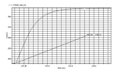
Figure 6.14: Amplifer settling time.
