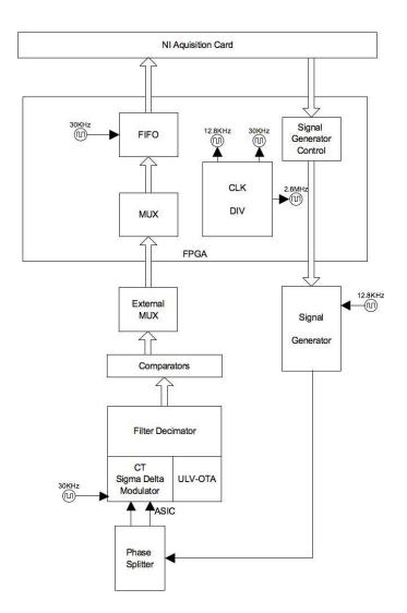
Figure 5.5: Modulator with FIR test and information configuration.
