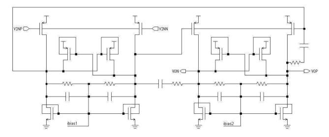
Figure 3.35: CT  $\Sigma\Delta$  Modulator
