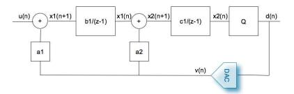
Figure 6.1: Second order DT  $\Sigma\Delta$  Modulator.
