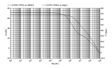
Figure 6.12: Open loop gain and phase.
