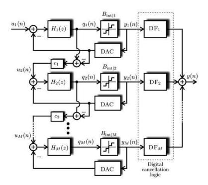
Figure 3.27: Cascade  $\Sigma\Delta$  modulators.
