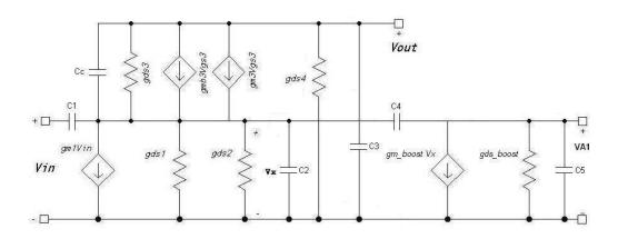
Figure 6.7: OTAs small signal model
