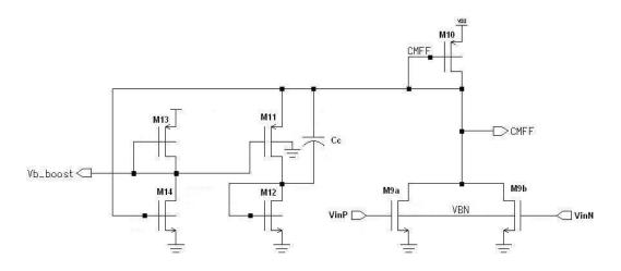
Figure 6.18: Common mode Feedforward circuit.
