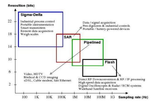
Figure 3.12: Trade-off between resolution and samplig rate.
