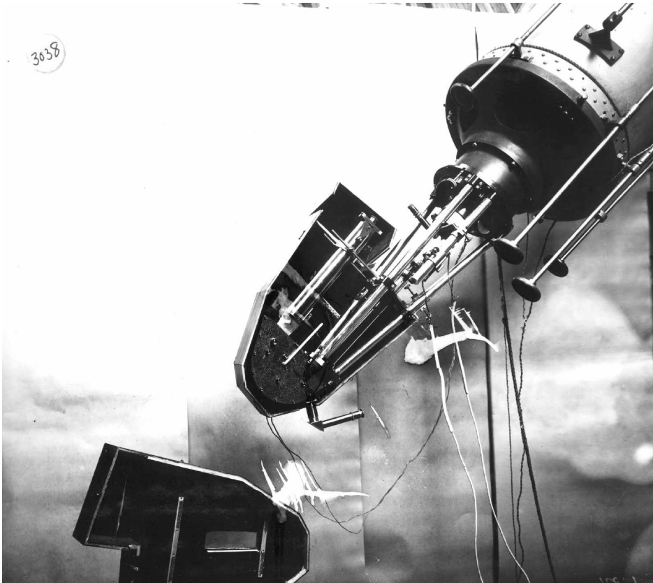
Figure 11: Le spectrographe initial de Slipher.
