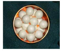
Figure 7.4: Axial view of the sample used in the microwave experiment.
