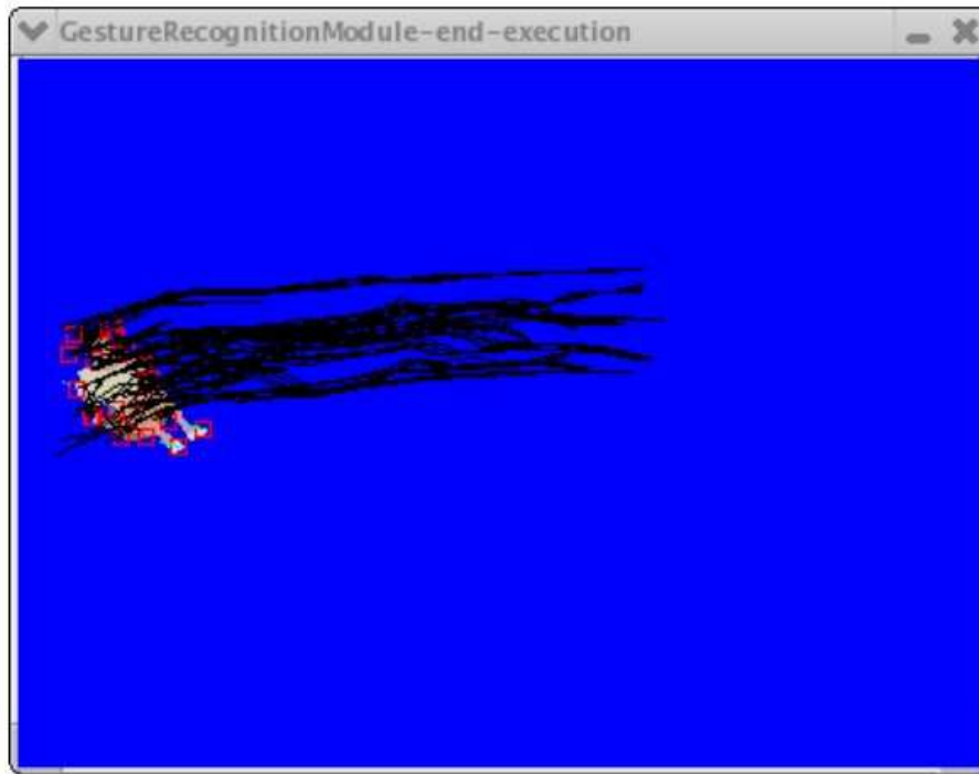
Figure 6.4: Synthetic data-set: red rectangles represent the tracked descriptors and the lines represent their trajectories.
