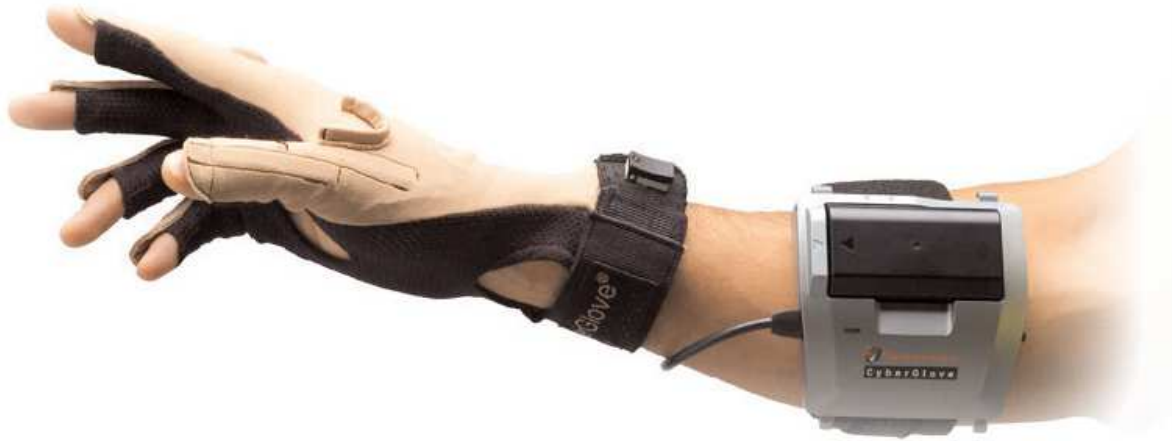
(a) Instrumented glove: Immersion cyberglove 2 is equipped with (1) potentiometers that measure rotation of joints with known length and rigid links and with (2) optic fibers which measure the amount of light passing through cables in order to measure bend.
