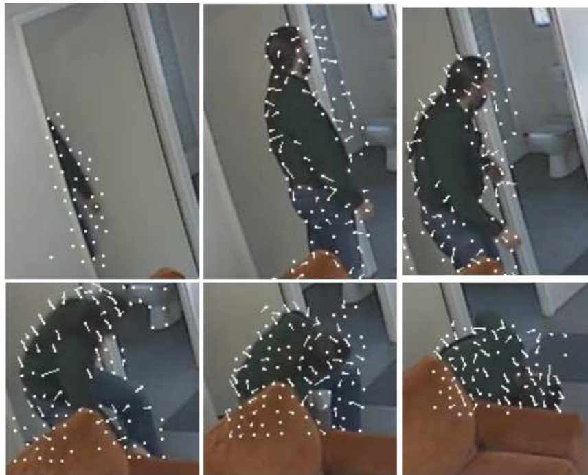
(a) Output of the KLT tracker: Each white line represents the history of motion of the correspondent corner point.
