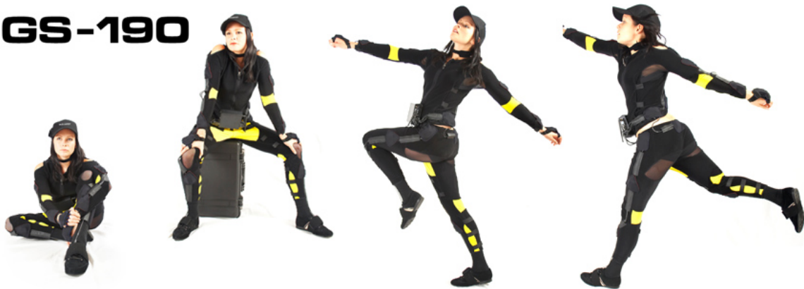
(b) Body suit: the Animazoo IGS-190 contains eighteen gyros for gesture recognition.
