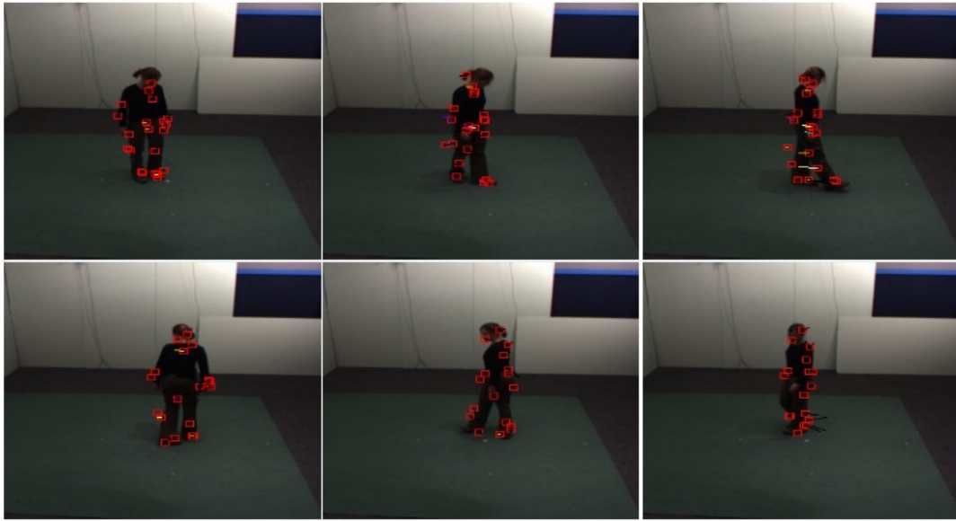
(a) Output of the proposed tracker with short term motion: only few descriptors and their correspondent motions are displayed.
