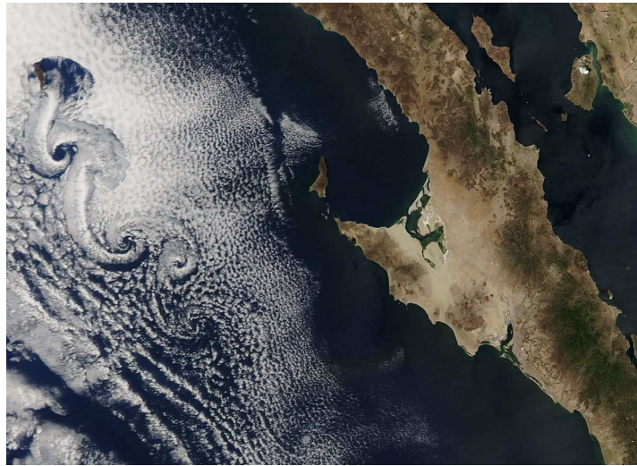
Figure 2.4: Von Karman vortex street over Baja California, Mexico (from U.S. Air Quality - the Smog Blog)
