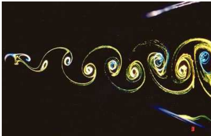
Figure 2.3: Vortex street at the back of a circular cylinder. Copyright ONERA 1996-2006
