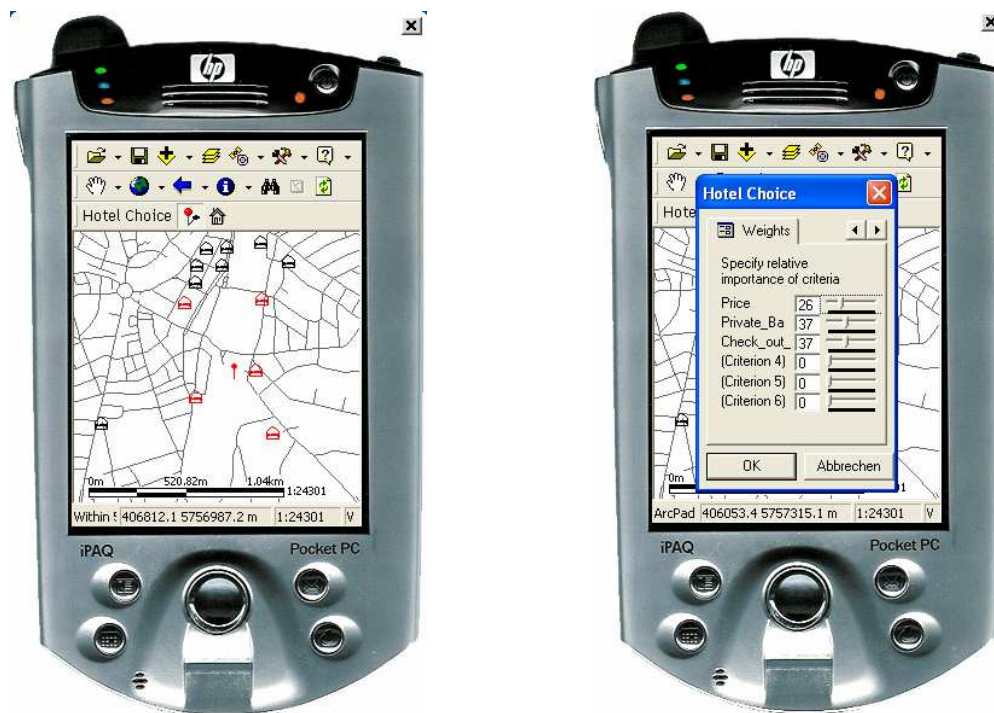
Figure 7.4: ArcPad desktop emulation on Pocket PC with GIS information, on the left part and with the definition of relative importance criteria weights by user, on the right part (from [101])
