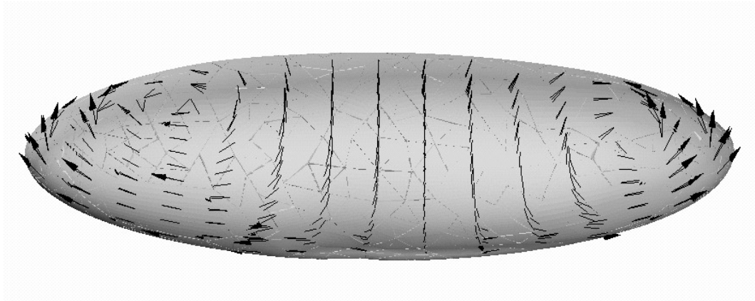
Figure 3.21: Simulation of the GBE with a hyperelastic model; the arrows represent the displacements field. The results show a high similarity with the ones with a Saint-Venant model.
