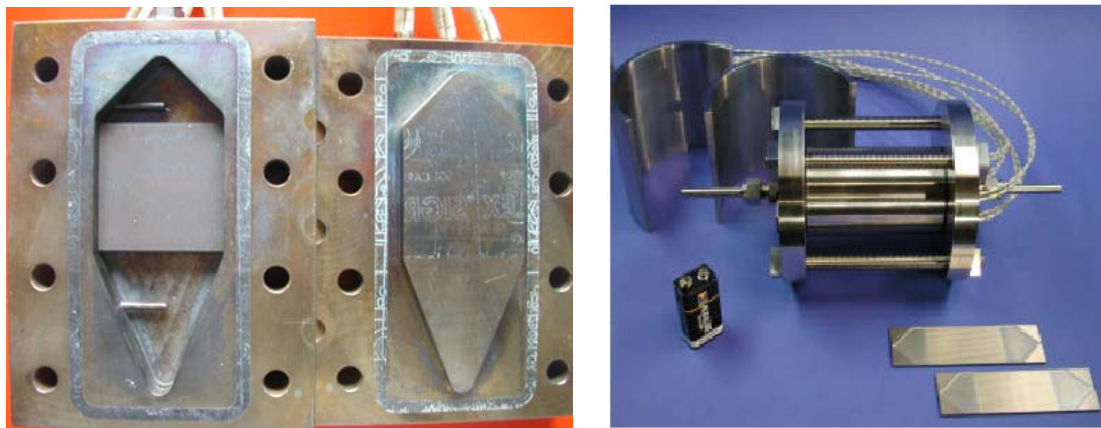
Fig 1 Micro-reactor housing used for ethanol oxidative steam reforming (left) and steam reforming (right)
