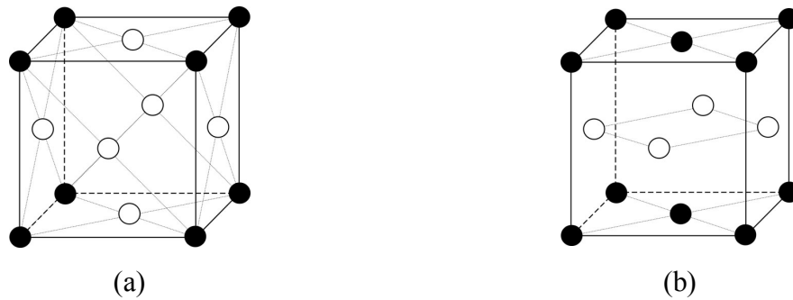
Figure 1.3. Distribution of Ni and Fe atoms on the sites of a fcc lattice for perfect atomic LRO substitutional superstructures:
