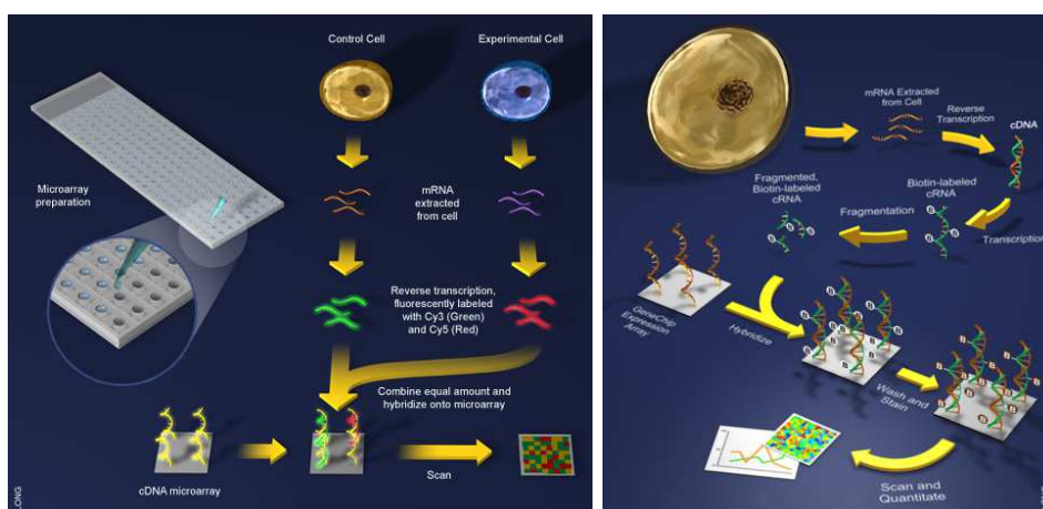
FIGURE 3. Comparison between spotted (left) and synthesized (right) microarrays, in the case of expression microarrays. Image Courtesy of The Science Creative Quarterly; artist: Jiang Long.
