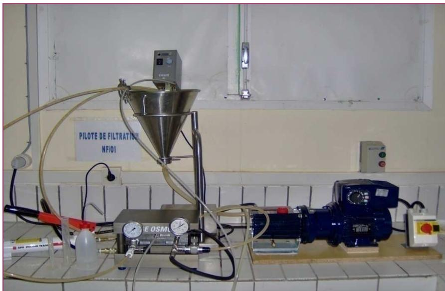
**Figure 20 :** Picture of the experimental set up used for salt mixture and real water experiments (Module SEPA CFII)
