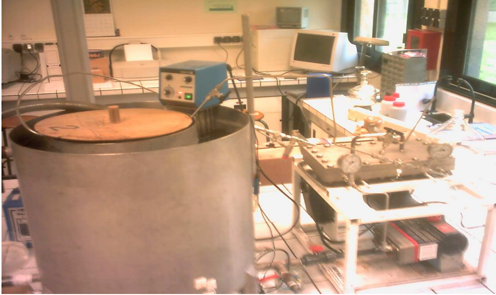
Figure 19: Picture of the experimental set up used for single salt experiments (Module SEPA II)
