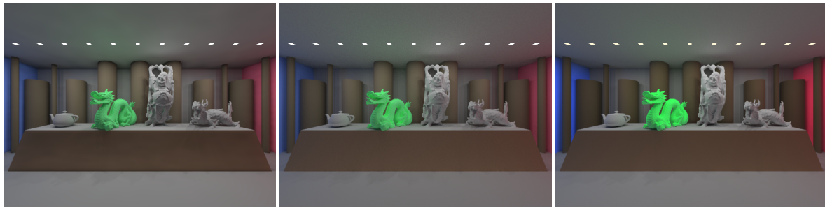
Fig. 3.11: Scene with mostly direct illumination case. 16 rays per pixel were used. 5 M photons shot. (left) Our technique with a 40 \times 50 \times 40 uncompressed grid (24.5 MB) used directly with a tricubic interpolation scheme. (Center) Photon mapping with Christensen’s Cache using 50 photons of the 5 M (124 MB) stored where used to precompute each irradiance sample. (right) Reference solution obtained by Path-Tracing with 1600 rays per pixel. The overall illumination is similar in all three techniques, however our much faster indirect illumination computation (51s vs. 5527s) strongly reduces the total rendering time (1341s vs. 6618s).
