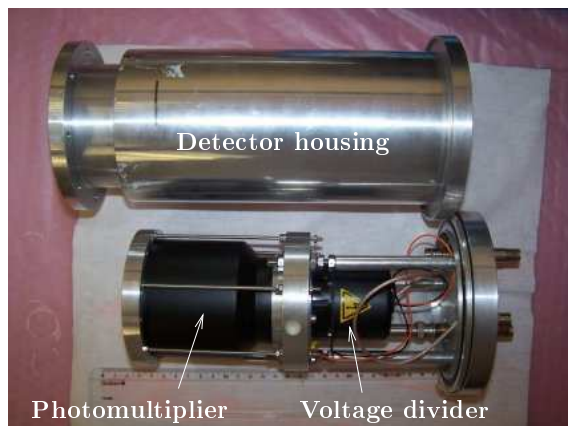
Figure 10.2: Set-up of the scintillator detectors.
