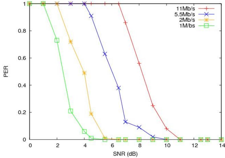
Fig 4.21 PER as a function of SNR
