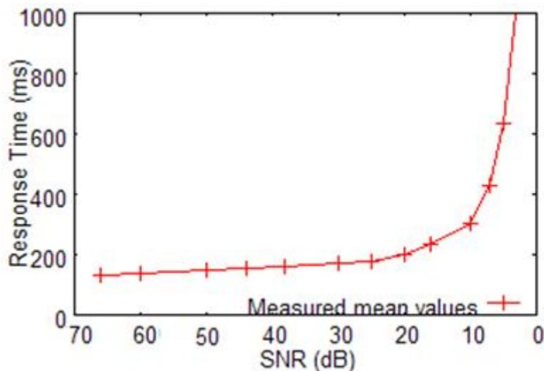
Fig 3.10 DHCP delay in terms of SNR
