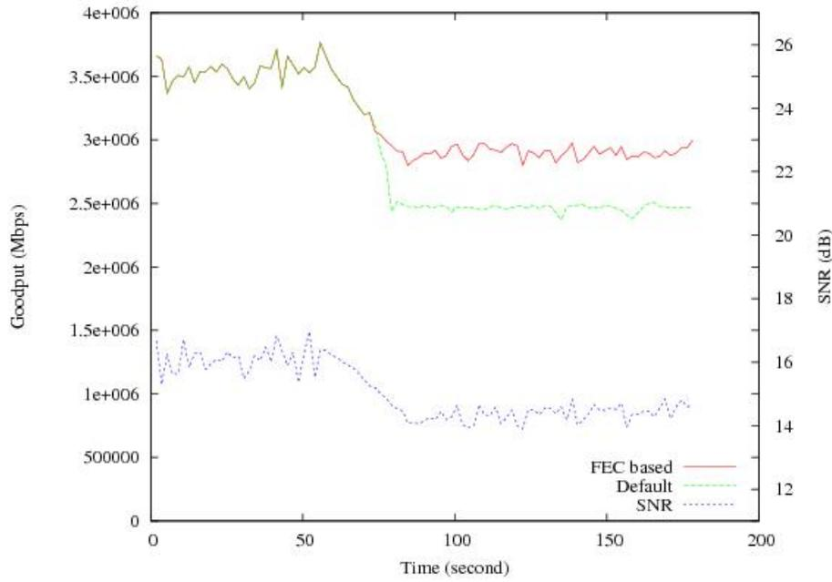
Fig.5.6 SNR evolution and Default/FEC based UL goodput
