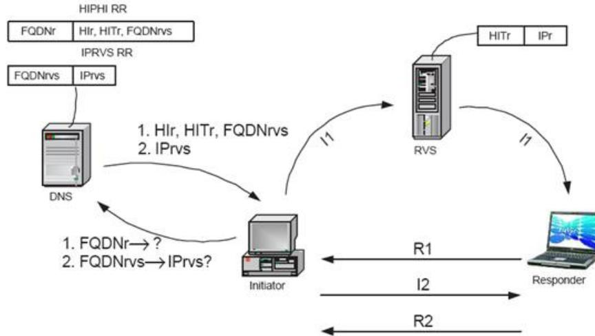
Fig 3.4-b Complete procedure of connection establishing via RVS
