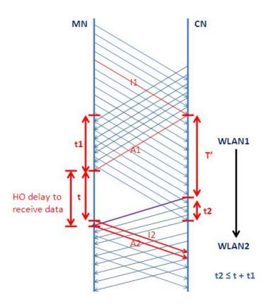
Fig 3.13 Sequence procedure of handover in case  $t2 \le t+t1$
