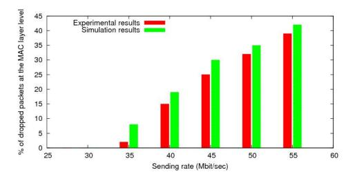
Fig 4.2 MAC layer overflow in UDP case
