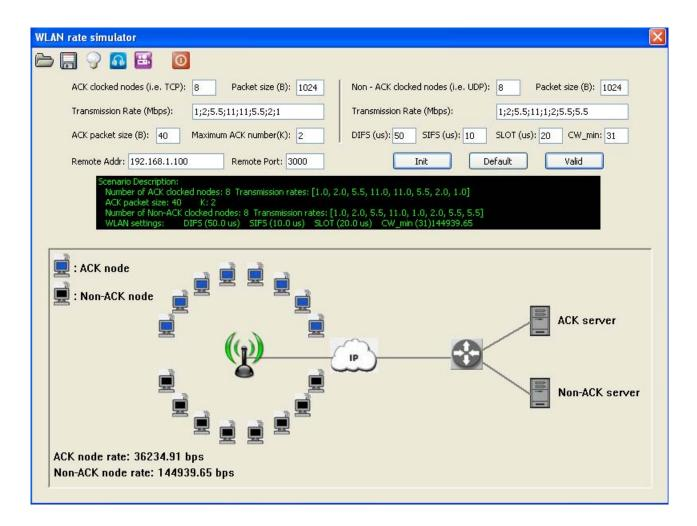
Fig 6.4 WLAN MAC bandwidth estimator
