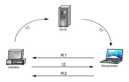
Fig 3.4-a Connection establishment via RVS
