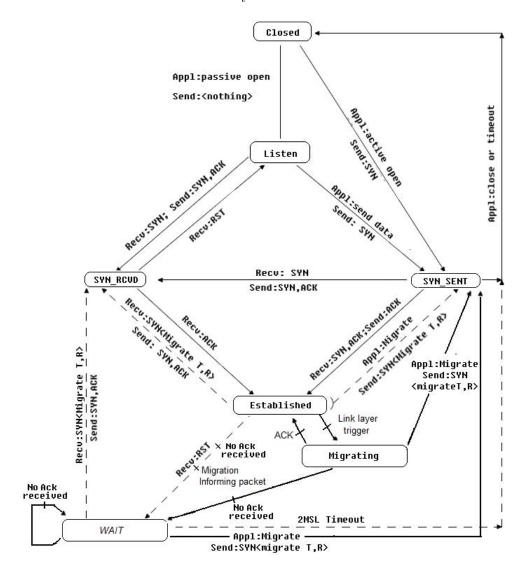
Fig 3.6-b State graph of continuous connection support
