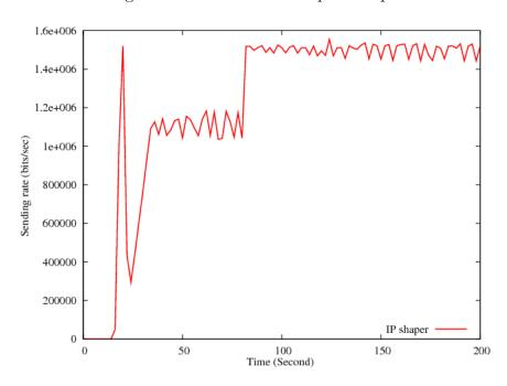
Fig 4.11-b TFRC rate IP shaper
