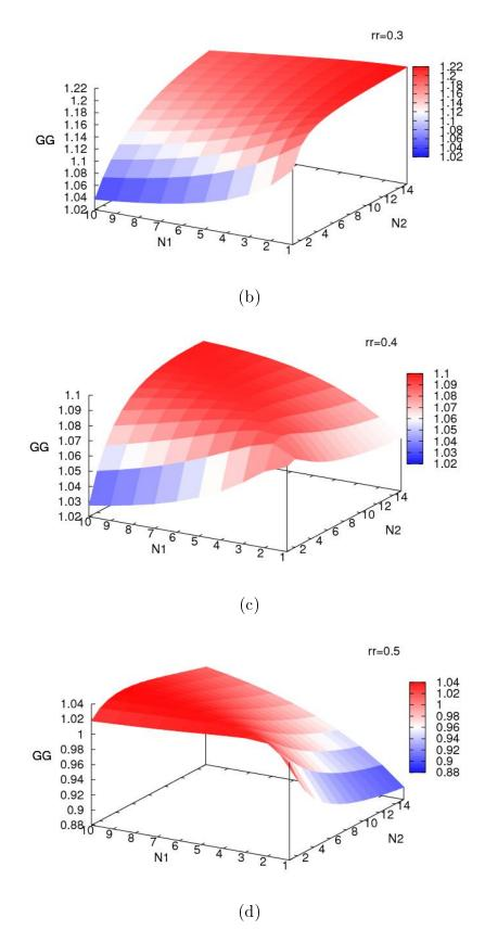
Fig 4.20 Global gain with a given rr as a function of N1 and N2
