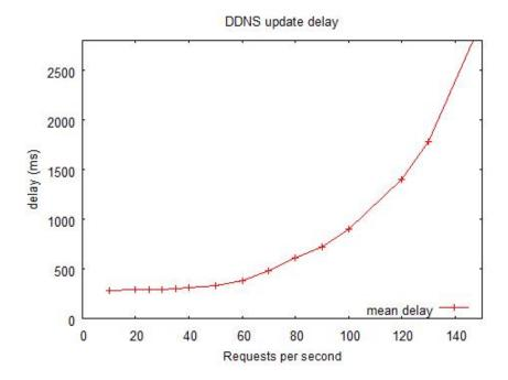
Fig 3.3 DDNS update delay in terms of request frequency
