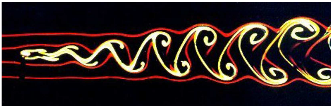
FIGURE 1.2: The Bénard-von Kármán vortex street behind a circular cylinder at Re = 65 (taken from Provansal et al. (2004)).
