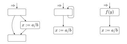
Figure 5.4: Three examples of incorrect code motion. Placing a computation of a/b at the program points marked by  $\Rightarrow$  can potentially transform a well-defined execution into an erroneous one.
