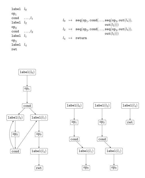
Figure 4.3: A code represented as a list of instructions (upper left), as a graph of instruction trees (upper right) and as a control-flow graph (lower left) along with its trees (lower right).
