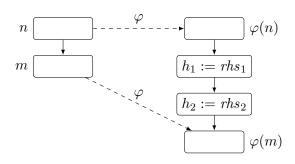
Figure 5.3: Effect of the transformation on the structure of the code
