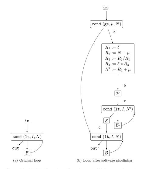
Figure 6.1: High level oveview of a software pipelining transformation
