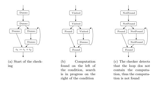
Figure 5.6: A few steps of the anticipability checking for computation  $t_1 + t_2$ . (Only the node at the way out of the graph holds the computation.)
