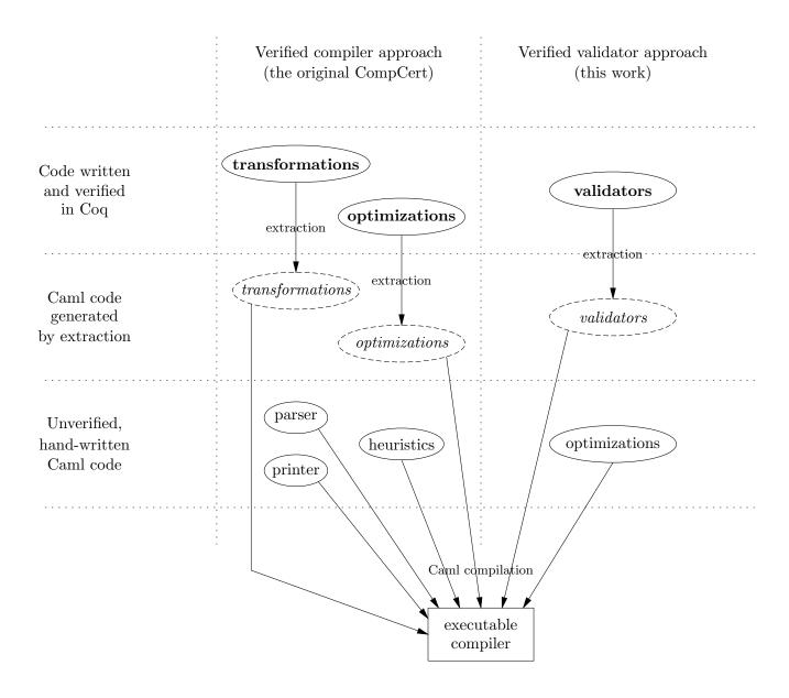
Figure 2.4: Compiler construction. On the left, the usual compiler construction process of Compcert. On the right, the compiler construction with verified validators and untrusted implementation of optimizations.
