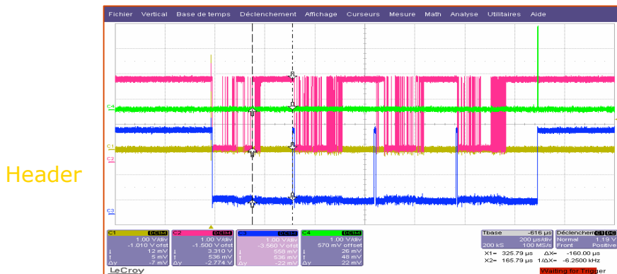
Figure 123: Four chips read-out sequentially, with the scheme described in §3.1.3. Each chip provides 128 events with 2 bits of data per event together with the BCID and chip header.
