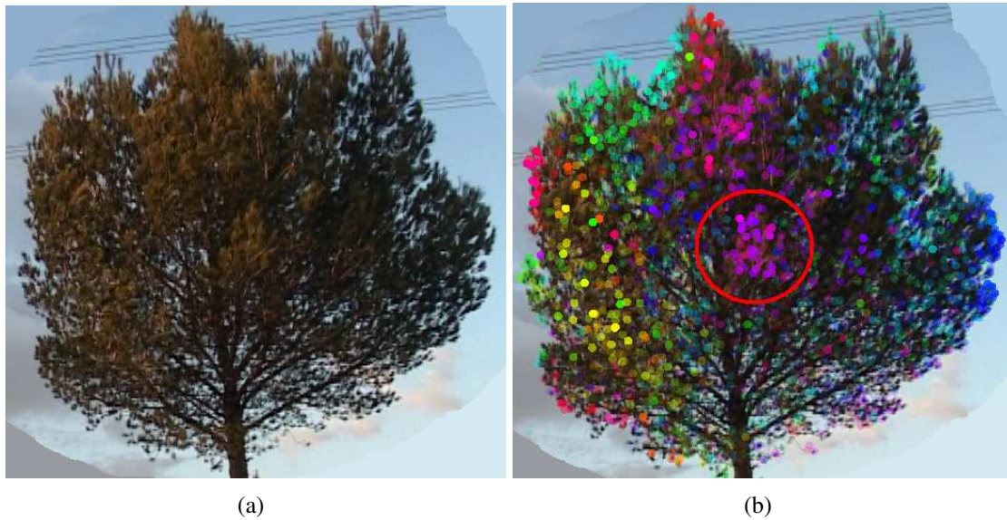
Figure 3.4: Superposition of motion information using speed to HSL mapping. (a) Original image from a video sequence. Structure is invisible . (b) With the motion information, the red circle indicates an emphasized structure.
