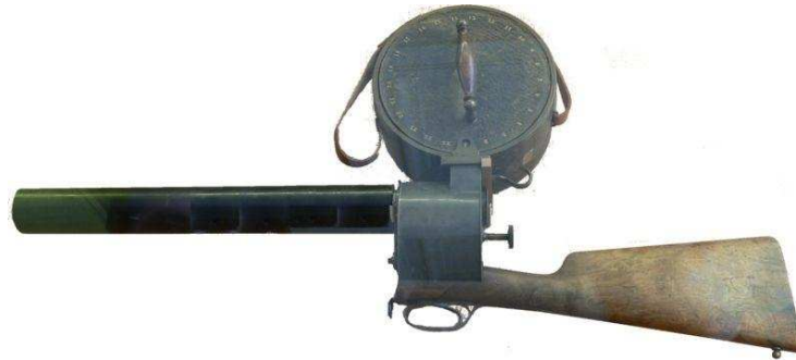
Figure 2.4: The chronophotographic gun design by Marey. A camera is mounted on a modified traditional gun where a photographic film is stored in the chamber. It allowed capturing up to twelve pictures by second.
