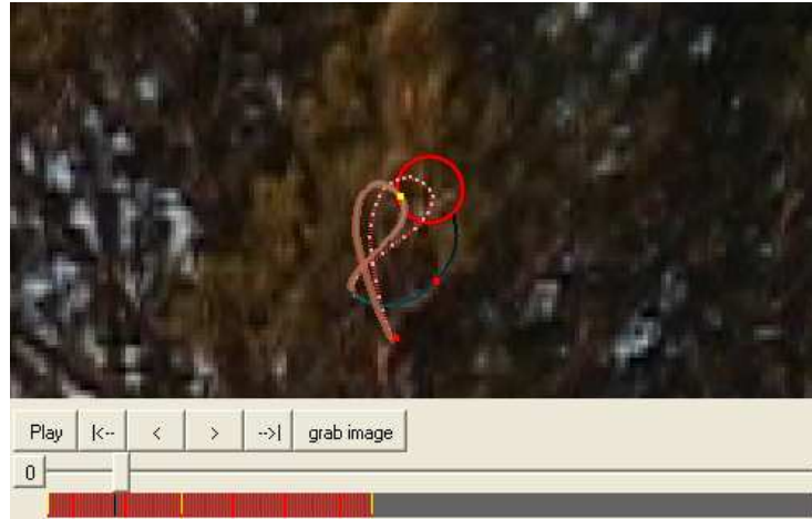
Figure 3.12: Spatial correction. The user corrects the position at one frame, and it is propagated along the motion curve. In light brown is the curve segment (initial curve) that is affected. The user has previously indicated the bound of this segment on one side. The other bound is the next key-frame (red dot). In light red curve with white points is the corrected motion curve, the points are the frames positions.
