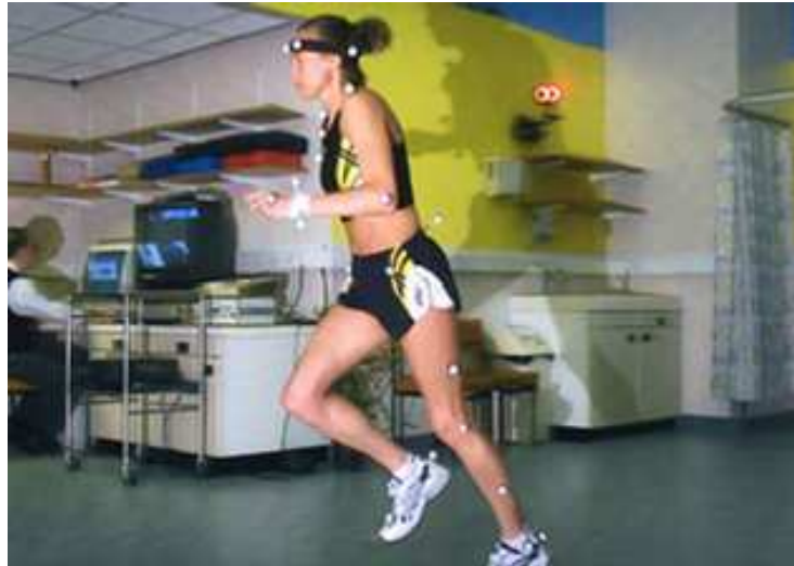
Figure 2.5: Tracking a human in motion using an infrared optical system. The subject has retroreflective markers set at specific parts of her body. A projector (red light at the top of the image) emits infrared light reflected by the markers. It is then detected in video sequences that film the subject.
