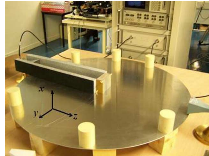
Fig. 9. The experiment setup for transmission measurement. Only the bottom plate is shown, top plate not shown for visibility purposes.
