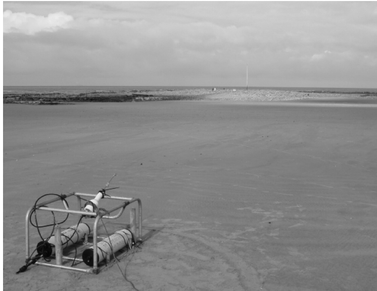
Figure 10.2: A photography of the ADV measuring device and its support, in the intertidal zone, before being submerged by the tide.
