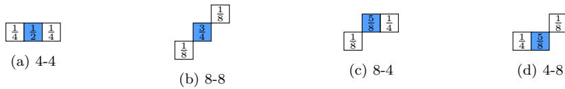
Figure 1.12: There are only four local masks appearing on an 8-connected line in the first octant.
