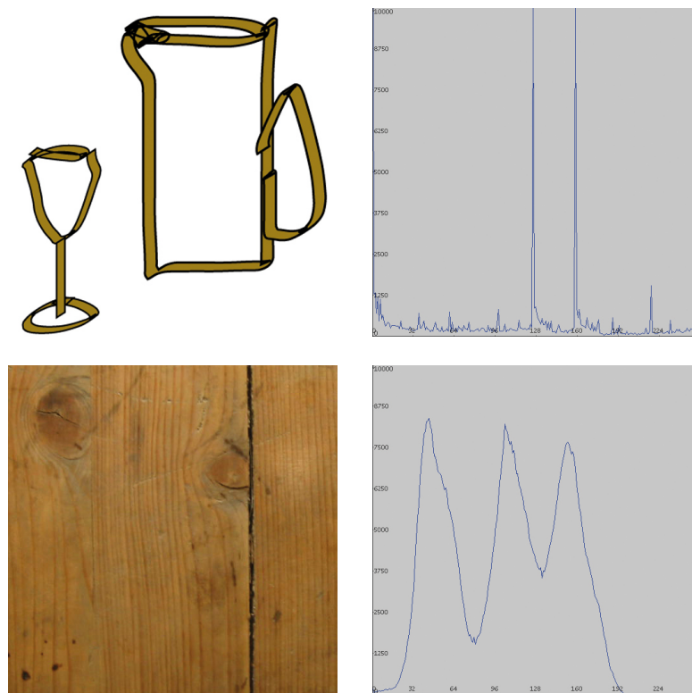
Figure 5.3: “Simple”(top) and “complex” (bottom) image textures and their respective histogram.
