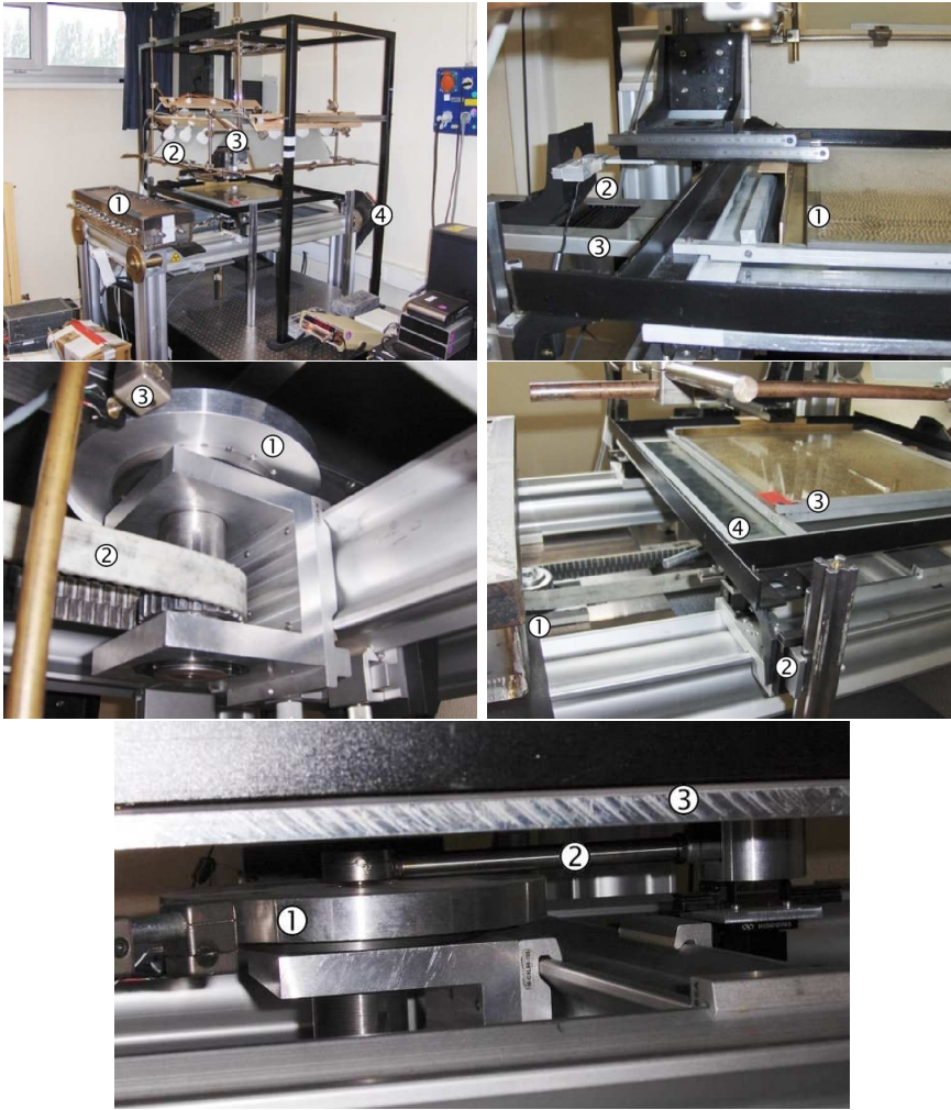
Figure 2.1: The experimental setup of the vibrating experiment. Top left: General view. One can see ① the counterweighting box full of lead, ② the lighting system, ③ the camera position and ④ the fixations of the experimental apparatus through the wall. Top right: View of ① the piston, ② the force sensor and ③ the translation platen. Middle left: View of ① the rotating device supporting the rod, ② the belt and ③ the trigger sensor. Middle right: View of ① the motor, ② the horizontality adjusting wheels, ③ the confinement cell and ④ the moving bottom plate. Bottom View of ① the rotating device stirring ② the rod. ③ The bottom plate oscillates at 10Hz with a 1cm amplitude.
