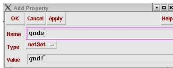
Figure A.13. Alimentation des prises substrats.
