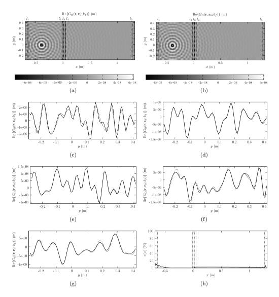
**Figure 5.6:** Real part of the Green's function of plate  $\Omega$  at 7 kHz. (a) Reference solution, (b) solution with virtual junction; (c-g) displacement field on vertical lines  $l_1$  to  $l_5$ ; ——, reference; · · · · · · , with virtual junction; (h) error from Eq. (5.17).
