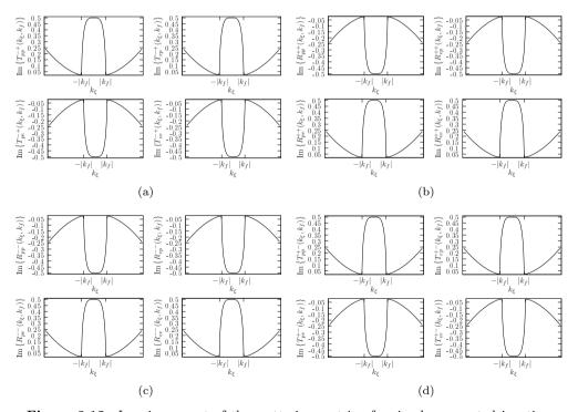
**Figure 3.12:** Imaginary part of the scattering matrix of a simply supported junction between two regions of an infinite plate. (a)  $T_{-+}$ , (b)  $R_{++}$ , (c)  $R_{--}$ , (d)  $T_{+-}$ .
