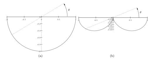
**Figure 3.8:** Real part of the first term  $R_{pp}$  of the reflection matrix for a simply supported edge (a) and a clamped edge (b), as a function of the angle of incidence of a propagating wave.
