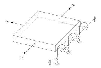
Figure 3.9: Schematic representation of an edge stiffener.
