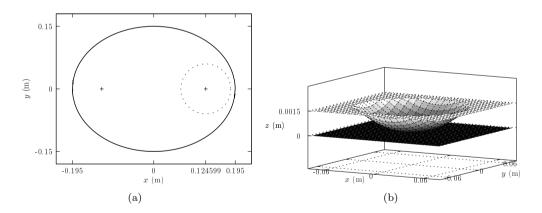
**Figure 7.13:** Elliptical plate with acoustic black hole profile at one of its foci. (a) Global view including dimensions in meters, (b) 3-D view of the top and bottom surfaces of the plate around the power-law pit. The radius of the pit is 6 cm, the maximum thickness of the plate is  $h_0 = 1.5$  mm and the thickness profile follows a quadratic law with distance, i.e.  $h(x) \sim x^4$ .
