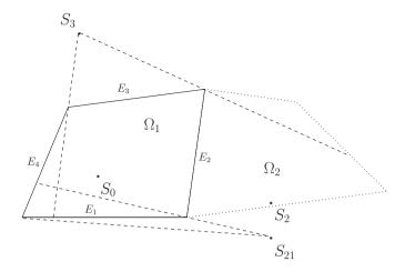
Figure 5.2: Example of visible and invisible image sources of plate  $\Omega_1$  (——) from a connected plate  $\Omega_2$  (·····).  $S_0$ , original source;  $S_2$ , image of  $S_0$  on edge  $E_2$ ;  $S_{21}$ , image of  $S_2$  on edge  $E_1$ ;  $S_3$ , image of  $S_0$  on edge  $E_3$ ; -----, validity zones of image sources. Source  $S_3$  is visible from a portion of both plates whereas source  $S_{12}$  is visible from a portion of plate  $\Omega_1$  but invisible from plate  $\Omega_2$ .
