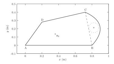
Figure 7.21: Polygonal plate with parabolic edge and acoustic black hole thickness profile.  $\mathbf{r}_0 = (0.36\,\mathrm{m}, 0.136\,\mathrm{m})$ , source; ..., acoustic black hole pit. The coordinates of the edges of the polygon are (in meters) A = (0,0), B = (0.8,0), C = (0.72,0.4) and D = (0.2,0.28). The centre of the parabolic edge is at 13.86 cm of the centre of BC and the centre of the black hole pit is at 6.36 cm of the centre of BC. The radius of the pit is 6 cm.
