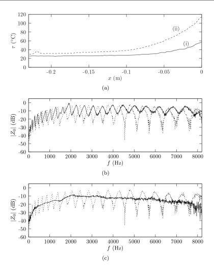
**Figure 8.7:** Measured temperature profiles and driving-point impedances for the uniform beam. (a) Temperature gradients; (b)  $\cdots$ , reference input impedance with no thermal load; ——, input impedance for temperature profile (i); (c)  $\cdots$ , reference input impedance with no thermal load; ——, input impedance for temperature profile (ii).
