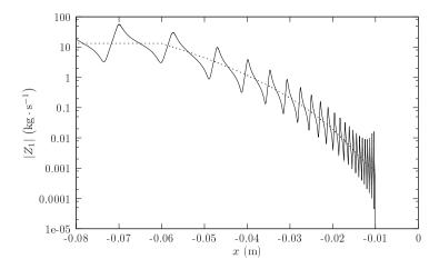
Figure 7.3: First term of the impedance matrix of a beam. ——, beam with black hole profile covered with a 10  $\mu$ m damping layer; · · · · · · , reference beam having a reflection matrix equal to zero.
