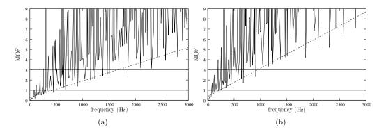
**Figure 2.9:** Modal Overlap Factor of the isosceles right triangular plate for two values of the structural damping ratio: (a)  $\eta = 3 \cdot 10^{-2}$ ; (b)  $\eta = 5 \cdot 10^{-2}$ . —, MOF; ----, least-squares fit of the local minimum.
