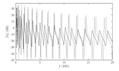
Figure 7.12: Simulated driving-point mobilities of a beam. ——, black hole beam; ....., uniform beam covered with damping layer in the black hole area; ----, uniform beam entirely covered with damping layer.
