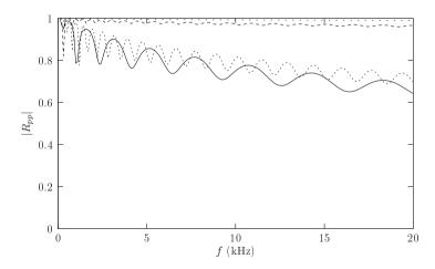
Figure 7.4: First term of the reflection matrix of a beam.  $\cdot \cdot \cdot$ , uniform beam covered with a 700  $\mu$ m damping layer ( $R_{20\text{kHz}}$ =0.985); -----, beam with black hole profile without damping layer ( $R_{20\text{kHz}}$ =0.97);  $\cdot \cdot \cdot \cdot \cdot$ , beam with black hole profile covered with 10  $\mu$ m of damping layer ( $R_{20\text{kHz}}$ =0.7); ——, beam with black hole profile covered with 700  $\mu$ m of damping layer ( $R_{20\text{kHz}}$ =0.62).
