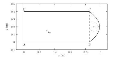
Figure 7.20: Rectangular plate with parabolic edge and acoustic black hole thickness profile.  $\mathbf{r}_0 = (0.2975\,\mathrm{m}, 0.148\,\mathrm{m})$ , source; ...., acoustic black hole pit. The coordinates of the edges of the rectangle are (in meters) A = (0,0), B = (0.85,0), C = (0.85,0.4) and D = (0,0.4). The centre of the parabolic edge is at 13.33 cm of the centre of BC and the centre of the black hole pit is at 5.83 cm of the centre of BC. The radius of the pit is 6 cm.
