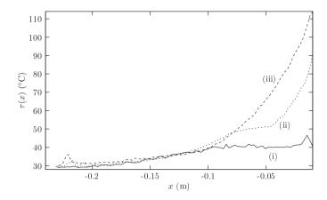
**Figure 8.3:** Measured temperature gradients on a uniform beam. Temperature at the bottom of the beam: ——,  $40.5 \,^{\circ}\text{C}$ ; ·····,  $90.3 \,^{\circ}\text{C}$ ; ····,  $114 \,^{\circ}\text{C}$ .
