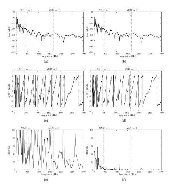
**Figure 2.13:** Frequency response of the isosceles triangular plate for two values of the truncation parameter: (a) modulus, (c) phase and (e) error for  $\gamma = 6.15$ ; (b) modulus, (d) phase and (f) error for  $\gamma = 30.74$ . —, exact solution; ----, AISM.
