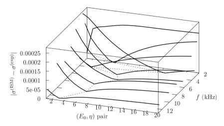
**Figure 6.8:** Search of optimum values of  $E_0$  and  $\eta$ . ———, difference between standard deviations of experimental and simulated driving point mobilities for each 1/3-octave band; ...., curve of minima across 1/3-octave bands.
