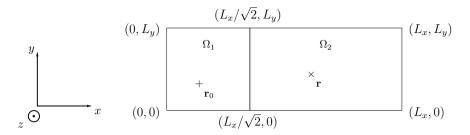
**Figure 5.4:** Assembly of two rectangular plates used for validation of the proposed approach, with  $L_x = 1$  m and  $L_y = 0.7$  m. The source position is  $\mathbf{r}_0 = (0.3 \,\mathrm{m}, 0.27 \,\mathrm{m})$ . —, plate edges; -----, virtual junction.
