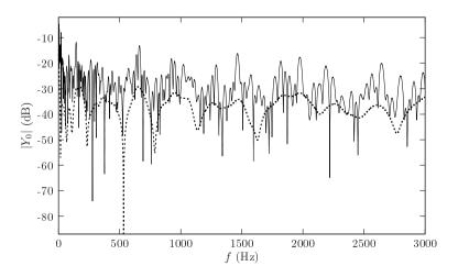
**Figure 7.26:** Simulated driving-point mobilities for a polygonal plate. ——, All edges free;  $\cdots$ , with a black hole edge.
