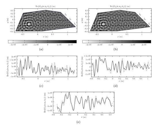
**Figure 5.8:** Real part of the Green's function for an assembly of two polygonal plates connected by a virtual junction. (a) Reference solution, (b) solution with virtual junction; (c-e) displacement field on horizontal lines  $l_1$  to  $l_3$ ; ——, reference; · · · · · · , with virtual junction.
