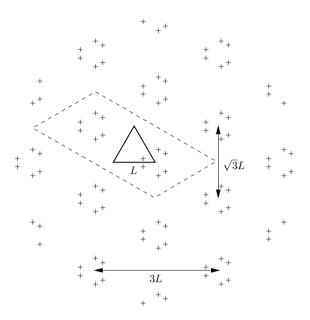
**Figure 2.6:** Image source cloud for the equilateral triangular plate. —, plate boundaries; +, sources; ---, elementary cell  $\mathcal{E}$ .
