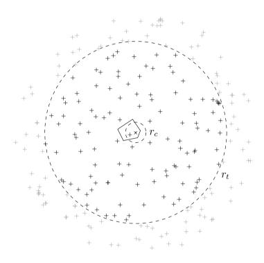
**Figure 2.7:** Example of image source cloud truncation for AISM. —, plate boundaries; ----, characteristic and truncation circles of radii  $r_c$  and  $r_t$  centered on the receiver; +, sources taken into account for AISM; +, ignored image sources.
