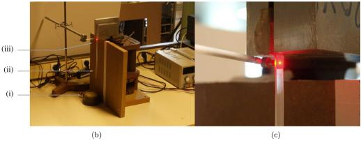
Figure 8.6: Experimental setup simultaneously measuring the temperature and driving-point response of a beam. (a) Schematic view, (b) photograph showing the heating resistance (i), the polymer beam (ii), the impact hammer and laser spot (iii), (c) zoom on the impact hammer and the laser spot.
