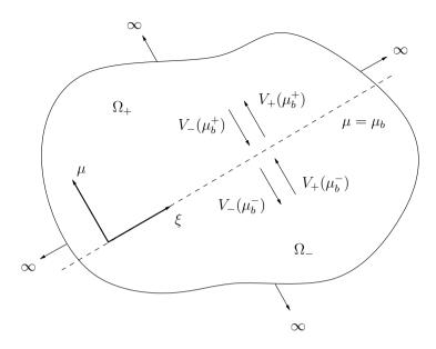
Figure 3.4: Junction between two semi-infinite plates  $\Omega^-$  and  $\Omega^+$ , located along line  $\mu = \mu_b$ . The different arrows represent the ingoing and outgoing waves at the junction.
