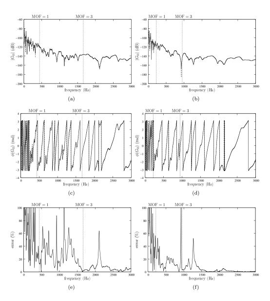
**Figure 2.10:** Frequency response function of the simply supported isosceles right triangular plate between source  $\mathbf{r}_0$  and receiver  $\mathbf{r}$ , calculated by modal expansion and by AISM for the truncation parameter  $\gamma=10.76$ , for two values of the structural damping ratio: (a) modulus, (c) phase and (e) error for  $\eta=3\cdot 10^{-2}$ ; (b) modulus, (d) phase and (f) error for  $\eta=5\cdot 10^{-2}$ . —, exact solution; ----, AISM.
