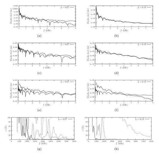
**Figure 4.12:** Modulus of the Green's function of the polygonal plate as a function of frequency computed by the proposed method  $(\cdots )$  and by FEM (----), for  $\eta = 0.07$  (left column) and  $\eta = 0.14$  (right column), at points (a,b)  $\mathbf{r}_1$ , (c,d)  $\mathbf{r}_2$  and (e,f)  $\mathbf{r}_3$ . (h,g) Error at points: -----,  $\mathbf{r}_1$ ; ------,  $\mathbf{r}_2$ ;  $\cdots \cdots$ ,  $\mathbf{r}_3$ .
