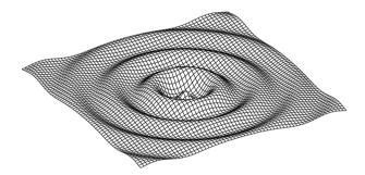
**Figure 1.3:** Real part of the Green's function of an infinite plate.
