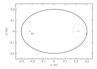
Figure 7.19: Elliptical plate with acoustic black hole thickness profile.  $\mathbf{r}_0 = (-0.2236\,\mathrm{m}, 0\,\mathrm{m})$ , source; ...., acoustic black hole pit. Semi-major and semi-minor axes are 30 cm and 20 cm, respectively. The radius of the black hole pit is 6 cm.
