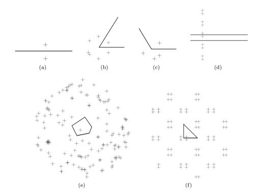
**Figure 1.4:** Examples of image source constructions for different two-dimensional geometries. (a) Semi-infinite domain, (b) sharp angle, (c) obtuse angle, (d) waveguide, (e) arbitrary polygon and (f) particular polygon.
