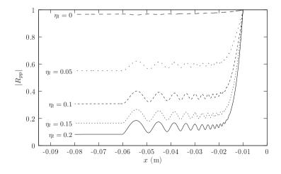
**Figure 7.9:** First term of the reflection matrix of the black hole beam for different values of the damping ratio of the damping layer, at frequency  $f = 20 \,\text{kHz}$ .
