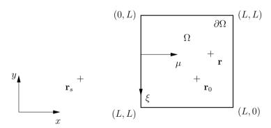
**Figure 6.1:** Square panel under consideration, with all edges free.  $\Omega$ , interior domain;  $\partial\Omega$ , boundaries;  $\mathbf{r}_0$ , source;  $\mathbf{r}$ , observation point. (x,y), global coordinate system;  $(\xi,\mu)$ , local coordinate system to an edge.
