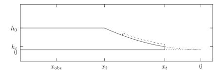
Figure 7.2: Side view of a beam with acoustic black hole profile and damping layer.
