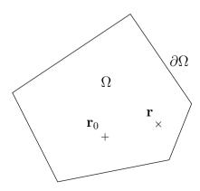
Figure 2.1: Polygonal plate with inside domain  $\Omega$  and boundaries  $\partial\Omega$ . +, source; ×, receiver.
