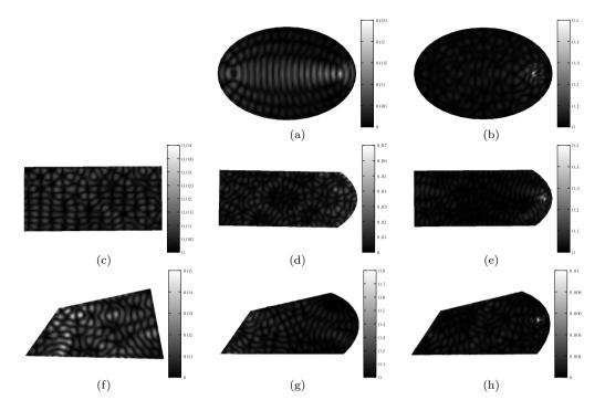
Figure 7.22: Magnitude of the experimental mobilities of different plates, in  $m \cdot s^{-1} \cdot N^{-1}$ . (a) Elliptical at 5220 Hz, (b) elliptical with black hole pit at 5220 Hz, (c) rectangular at 3289 Hz, (d) rectangular with parabolic edge at 3289 Hz, (e) rectangular with black hole parabolic edge at 3289 Hz, (f) arbitrary polygonal plate at 3289 Hz, (g) arbitrary polygonal plate with parabolic edge at 3289 Hz and (h) arbitrary polygonal plate with black hole parabolic edge at 3289 Hz.
