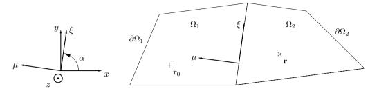
**Figure 5.1:** Assembly  $\Omega$  of two plates  $\Omega_1$  and  $\Omega_2$ .  $\mathbf{r}_0$ , source,  $\mathbf{r}$ , observation point, (x, y), global coordinate system,  $(\xi, \mu)$ , local coordinate system for computing reflection or transmission at a boundary.
