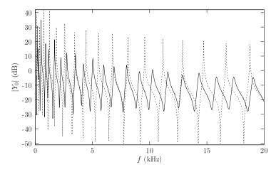
**Figure 7.11:** Simulated driving-point mobilities of a beam. ——, black hole beam; ....., untreated uniform beam.
