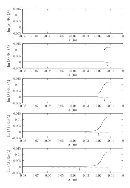
**Figure 7.7:** Ratio of the imaginary part to the real part of the wavelength for different lengths of the damping layer. The dotted line represents the portion of the beam that is covered with the damping layer.
