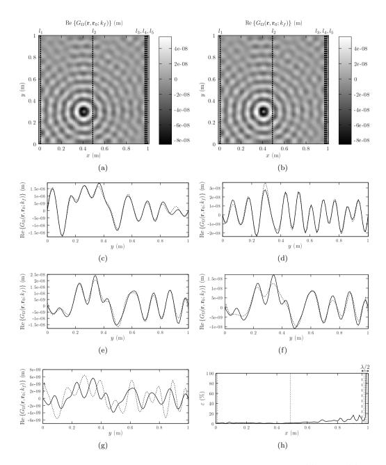
**Figure 4.7:** Amplitude of the Green's function for the square plate. (a) Exact; (b) proposed method; (c) to (g) displacement field on vertical lines  $l_1$  to  $l_5$ ; ——, exact; …—, proposed method.
