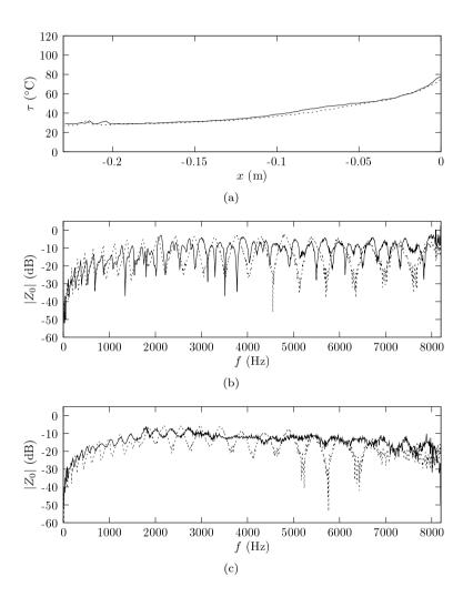
**Figure 8.8:** Comparison between uniform and varying-thickness beams. (a) Temperature profiles: -----, uniform beam; ——, beam with power-law thickness. (b) Input impedances of the uniform beam, (c) input impedances of the power-law beam. ······, with no thermal load; ——, with temperature profiles of (a).
