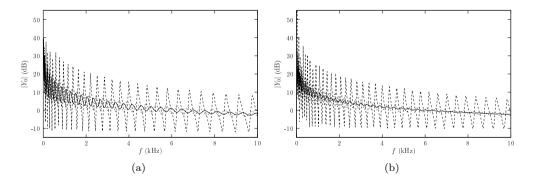
**Figure 8.5:** Driving-point mobilities for different temperature gradients. (a) Uniform beam, (b) beam with power-law thickness profile. ...., no thermal load; ----, temperature profile (i) of Fig. 8.3; ——, temperature profile (iii) of Fig. 8.3.
