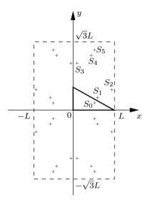
**Figure 2.16:** Elementary cell of the half-equilateral triangular plate. Six sources, denoted  $S_i$  (i = 0, ..., 5) and located at  $(x_i, y_i)$ , are necessary to describe this cell.
