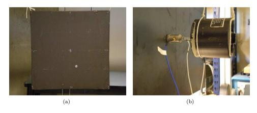
**Figure 6.3:** Photography of the damped panel under test. (a) Front view, (b) rear view.
