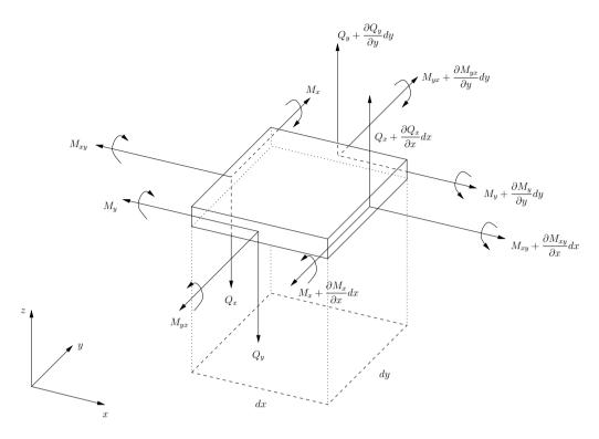
**Figure 1.1:** Surface element of a thin plate with applied forces and moments. After Graff [34].
