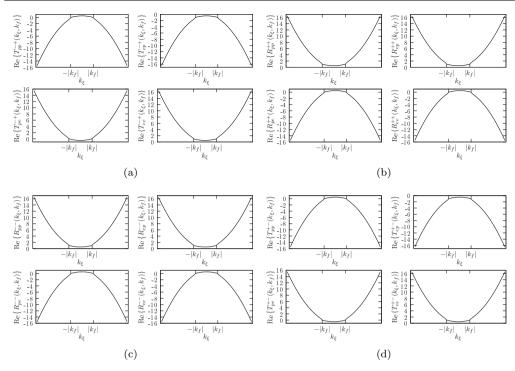
**Figure 3.11:** Real part of the scattering matrix of a simply supported junction between two regions of an infinite plate. (a)  $\mathbf{T}_{-+}$ , (b)  $\mathbf{R}_{++}$ , (c)  $\mathbf{R}_{--}$ , (d)  $\mathbf{T}_{+-}$ .
