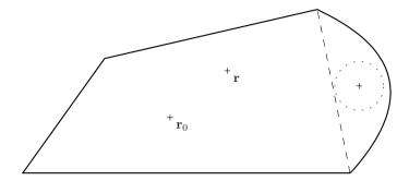
**Figure 7.17:** Polygonal plate with parabolic edge and acoustic black hole thickness profile.  $\mathbf{r}_0$ , source;  $\mathbf{r}$ , observation point;  $\cdots$ , acoustic black hole pit; ----, virtual boundary separating the polygonal plate from the black hole zone.
