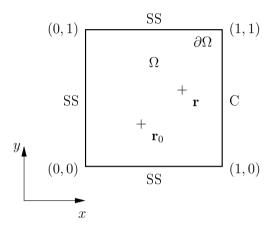
Figure 4.6: Square plate with three simply supported (SS) edges and one clamped (C) edge.
