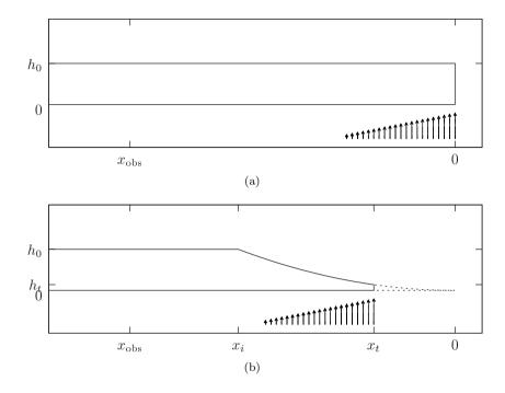
**Figure 8.1:** Side view of a beam exposed to a temperature gradient. (a) Uniform beam, (b) beam with power-law varying thickness (——, real profile with initial and truncation distances  $x_i$  and  $x_t$ ; ...., ideal black hole profile). The arrows indicate the thermal load.
