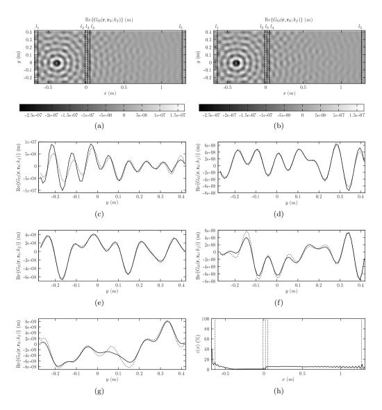
**Figure 5.5:** Real part of the Green's function of plate  $\Omega$  at 3 kHz. (a) Reference solution, (b) solution with virtual junction; (c-g) displacement field on vertical lines  $l_1$  to  $l_5$ ; ——, reference; …, with virtual junction; (h) error from Eq. (5.17).
