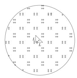
Figure 2.8: Image source cloud of the isosceles right triangular plate, for the truncation parameter  $\gamma = 10.76$  ( $r_t = 4.95$  m), containing 154 sources.
