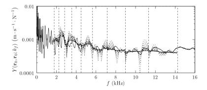
**Figure 6.7:** Experimental and simulated driving point mobilities with estimated Young's moduli for each 1/3-octave band. ———, experimental; · · · · · · , ISM for a damping ratio from  $\eta = 0.01$  to  $\eta = 0.2$ ; -----, 1/3-octave-band limits.
