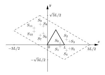
**Figure 2.17:** Elementary cell of the equilateral triangular plate. Twelve sources, denoted  $S_i$  (i = 0, ..., 11) and located at  $(x_i, y_i)$ , are necessary to describe this cell.
