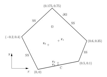
**Figure 4.8:** Polygonal plate for comparison of the proposed approach to FEM with clamped (C) and simply supported (SS) boundaries.  $\mathbf{r}_0 = (0.125, 0.3)$ , source;  $\mathbf{r}_1 = (0.245778, 0.350778)$ ,  $\mathbf{r}_2 = (0.245778, 0.073775)$  and  $\mathbf{r}_3 = (0.245778, 0.058386)$ , observation points. Coordinates are in meters.
