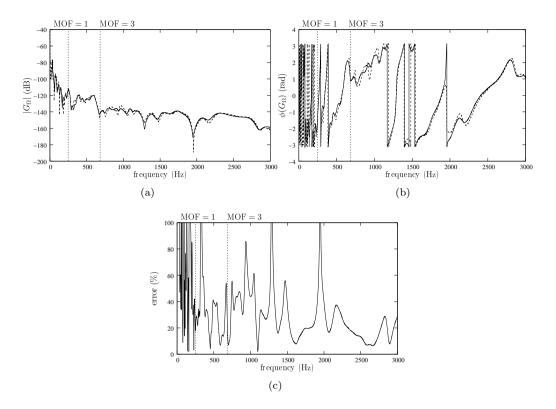
**Figure 2.12:** ISM and FEM simulations for the arbitrary polygonal plate of Fig. 2.11 for the damping ratio  $\eta = 0.07$ . (a) modulus, (c) phase and (e) error. —, FEM solution; ----, AISM.
