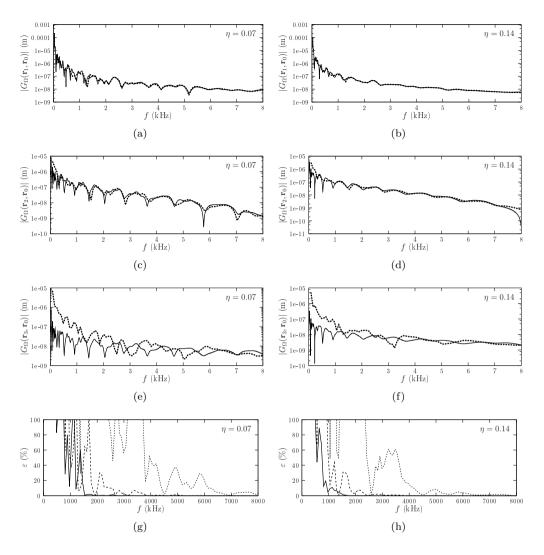
**Figure 4.9:** Modulus of the Green's function of the polygonal plate as a function of frequency computed by the proposed method  $(\cdots )$  and by FEM (---), for  $\eta = 0.07$  (left column) and  $\eta = 0.14$  (right column), at points (a,b)  $\mathbf{r}_1$ , (c,d)  $\mathbf{r}_2$  and (e,f)  $\mathbf{r}_3$ . (h,g) Error at points: ----,  $\mathbf{r}_1$ ; -----,  $\mathbf{r}_2$ ;  $\cdots \cdots$ ,  $\mathbf{r}_3$ .
