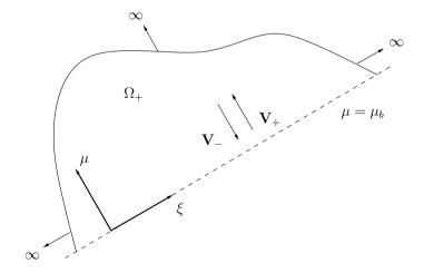
Figure 3.3: Edge of a semi-infinite plate  $\Omega^+$ , located along line  $\mu = \mu_b$ .  $\mathbf{V}_+$  and  $\mathbf{V}_-$  respectively represent the wave vectors associated to incident and reflected fields.
