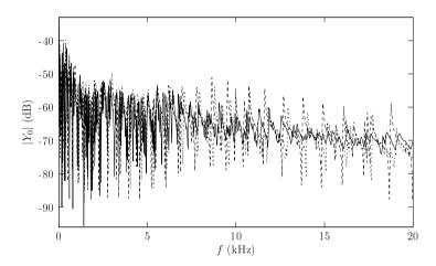
Figure 7.16: Measured driving-point mobilities of elliptical plates. ——, black hole plate; -----, uniform plate covered with absorbing resin in the black hole area; ······, uniform plate entirely covered with absorbing resin.
