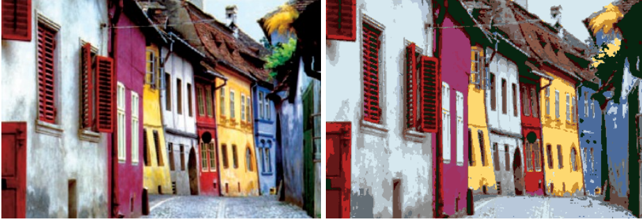
Figure IV.3 – Distance-based mean-shift followed by k-Means clustering on the point cloud made of LUV colors of the pixels of the picture on the right.
