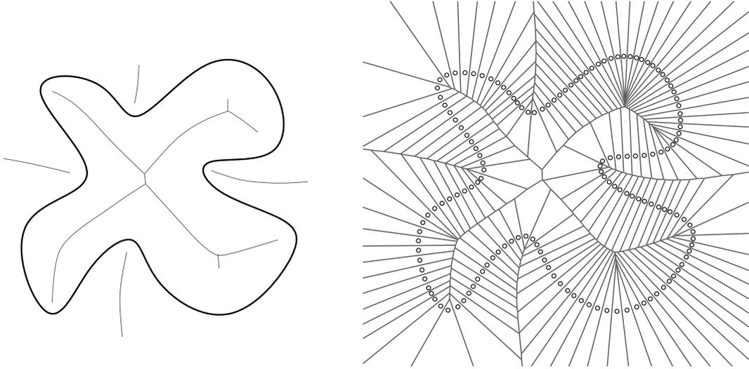
**Figure I.1** – Medial axis of a curve  $C$  in the plane, and Voronoi diagram of a point cloud  $P$  sampled on the curve. Notice that while  $P$  and  $C$  are Hausdorff close, their respective medial axes are very different.
