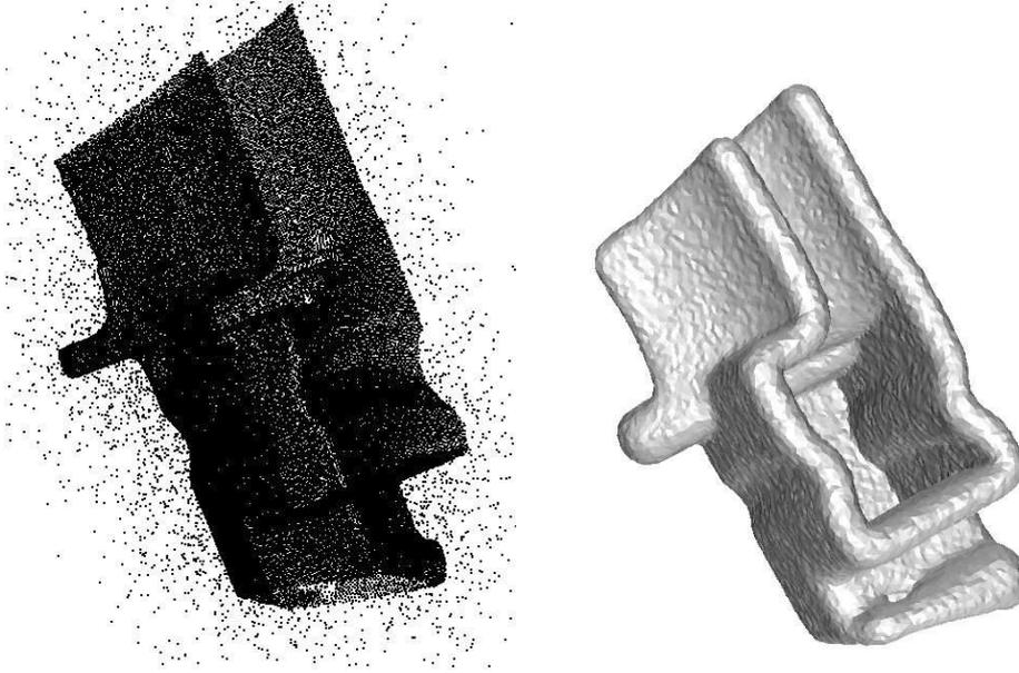
**Figure IV.2** – On the left, a point cloud sampled on a mechanical part (blade) to which 10% of outliers have been added — the outliers are uniformly distributed in a box enclosing the original point cloud. On the right, the reconstruction of an isosurface of the distance function  $d_{\mu_C, m_0}$  to the uniform probability measure on this point cloud (obtained by using the CGAL Surface Mesher).
