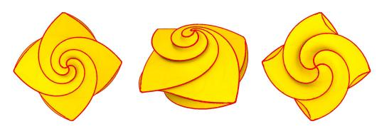
**Figure III.1** – Features (in red) computed by our algorithm from a point cloud sampling of the surface in yellow.
