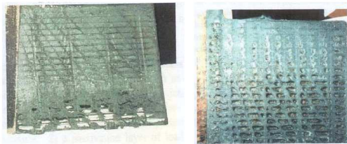
Figure 30: Stratification effect on a positive plate: softening and shedding of the active material at the bottom of the plate [48].
