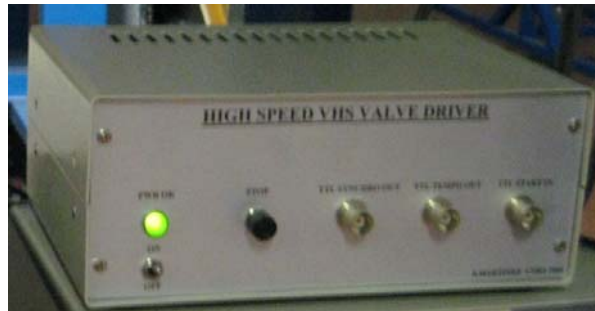
Figure 4.5 High Speed VHS Valve Driver (IUSTI, S. Martinez)
