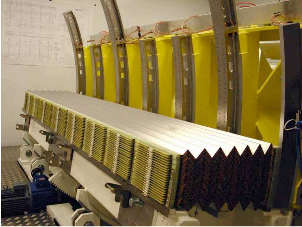
Figure 3.3: View of a module of the accordion calorimeter of the ATLAS barrel during assembly.
