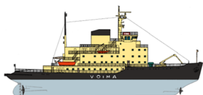
VOIMA 1954 Shaft output 10200 kW (modernised 1979)
