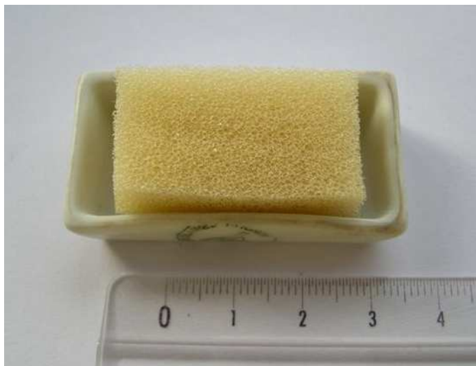
Figure 2-12 Tubular furnace sample. The mass is around 110 mg
