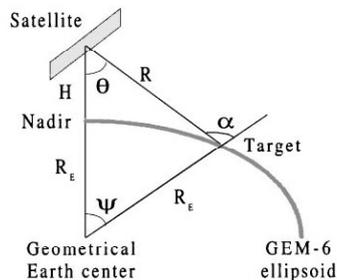
Fig. 1. Acquisition geometry.
