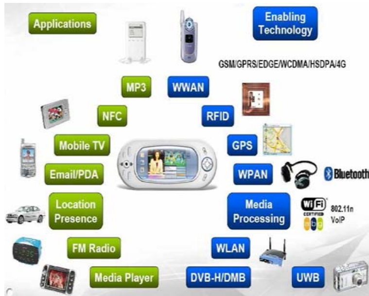
Fig. 1.1. Different mobile applications and their enabling technologies [1].
