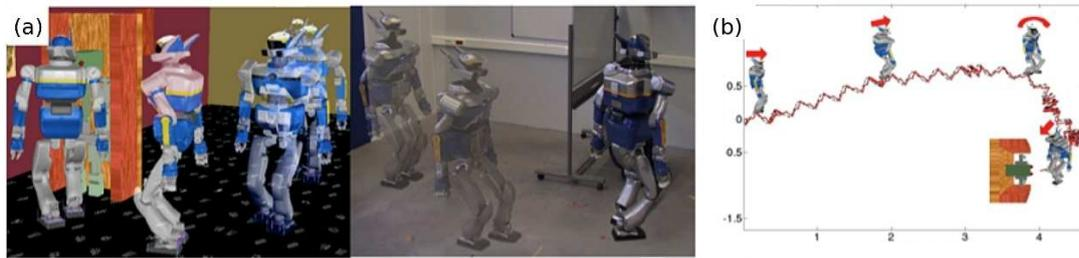
Figure 5.15: Extracted with author permission from [Sree09]. (a) HRP2 being maneuvered through space to find distant, hidden objects. (b) Plot of head position (solid line) and center of mass (CoM) position (dotted line) during motion. The zig-zag motion of the head and CoM position was due to the user alternatively looking left and right at every step.
