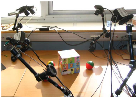
Figure 7.2: The 5-camera setup used for the experiments. The stereo pair (top-left) is used for initialization.
