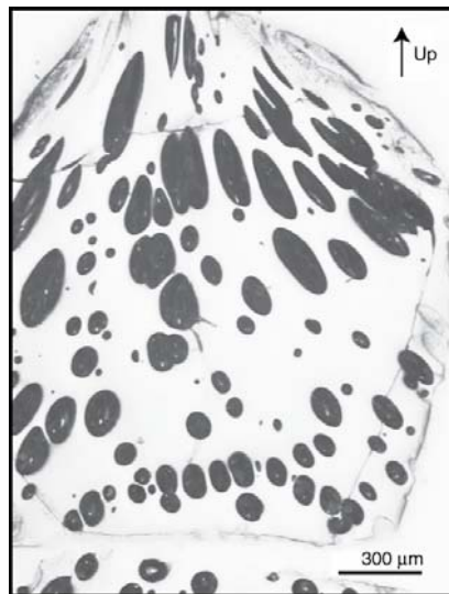
Figure 2 Reflected light microphotograph of the upper 2 mm of run G318 (Table 2). Bubbles are deformed because the melt has been squeezed up in the capsule headspace by volumetric expansion. Note that this type of extrusion occurs in both open and closed degassing conditions. This open degassing sample illustrates the catalyzing effect of shear on coalescence. Note that the large, coalesced bubbles are restricted to the upper half of the photograph, where the shear was highest.
