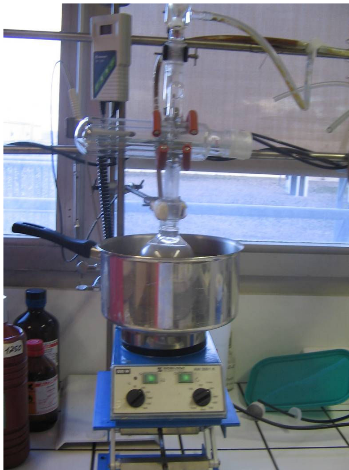
Fig. 6-7. Installation for bulk polymerisation
