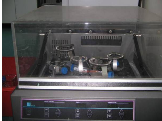
Fig. 6-19. Installation for pellets stirring – calcification tests.
