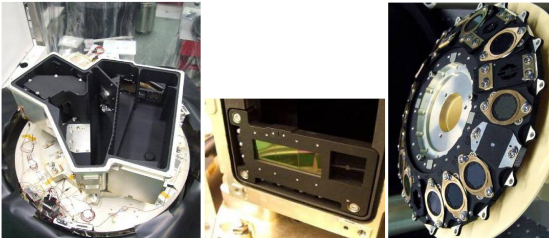
Figure 10.9: Left: the MIRIM open box. Middle: the focal plane, with the four coronagraph masks (one Lyot and three 4QPMs). Right: the filter wheel, providing the broad-band filters for imaging, the coronagraph filters, the double prisms for the LRS, and the alignment lens.
